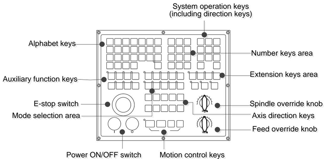
Fig. 1-12 Front view of WH108C operation panel
