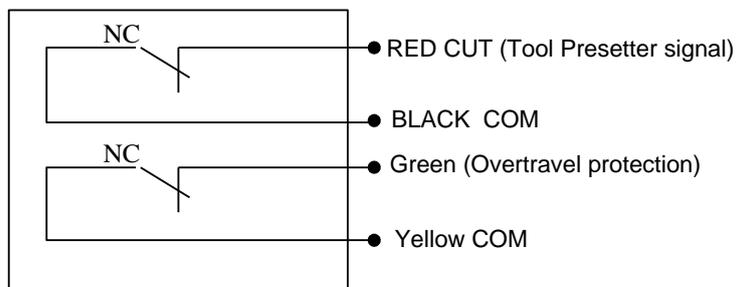
Fig. 3-23 Electrical Wiring Diagram of A WEIHONG Tool Presetter
