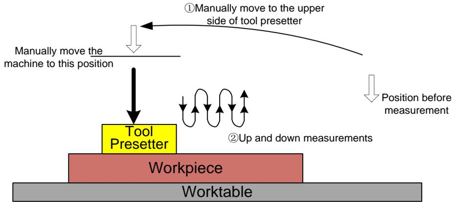
Fig. 3-30 The Process of Mobile Calibration without Encoder Feedback Function
