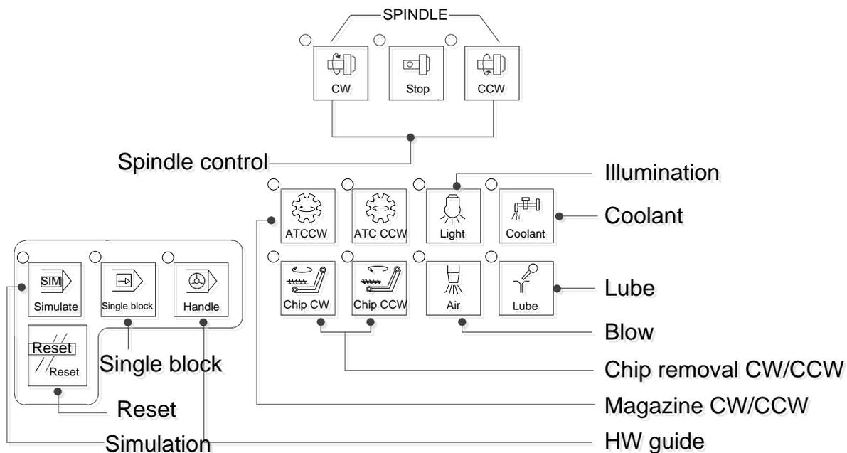
Fig. 1-8 Auxiliary function keys
