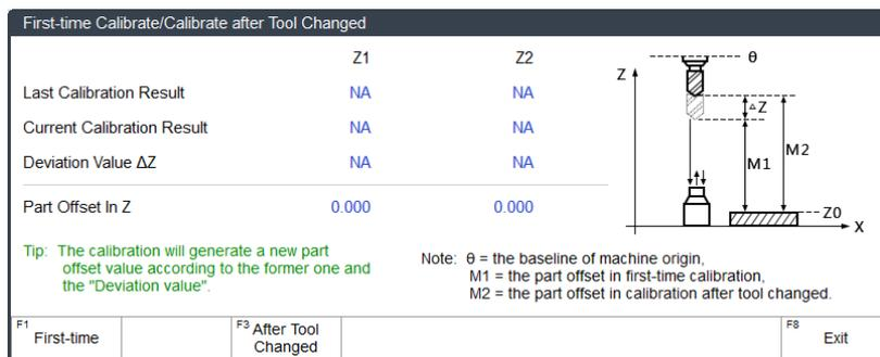
Fig. 4-6 First time/after TC calibration of multi-Z software
