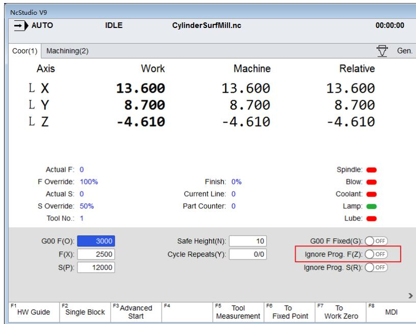
Fig. 3-44 Parameters Setting Zone-feedrate Setting
