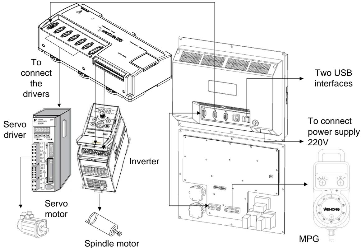
Fig. 1-20 Overall connection diagram of NK300CX-V
