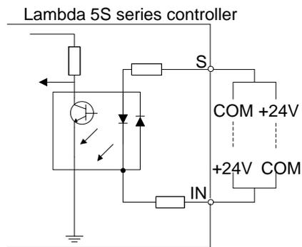
Fig. 2-1 Connection of binary input and mechanical switch
