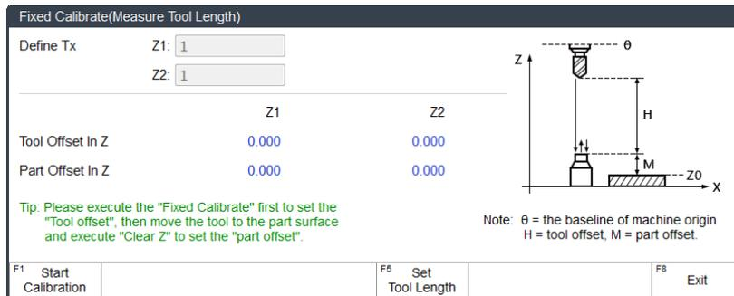
Fig. 4-5 Fixed calibration dialog box of multi-Z software
