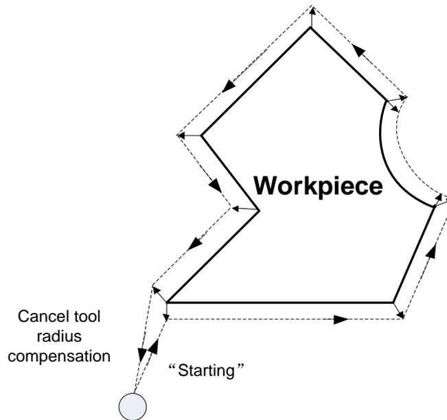
Fig. 3-51 Schematic Diagram for Tool Radius Compensation
