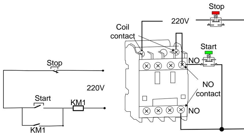
Fig. 2-6 Wiring diagram of electrical switch on operation panel
