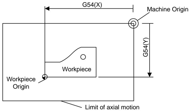
Fig. 3-35 The Relationship of Work Offset and Machine Coordinate System
