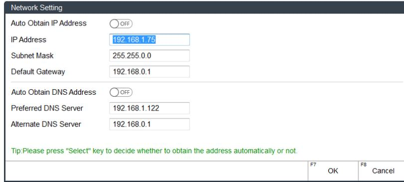
Fig. 3-81 Manually Set IP Address
