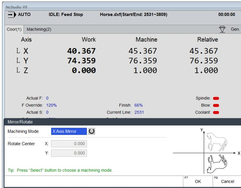
Fig. 3-94 Mirror and Rotate Setting on the Main Interface
