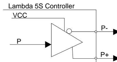
Fig. 2-4 Pulse command output circuit
