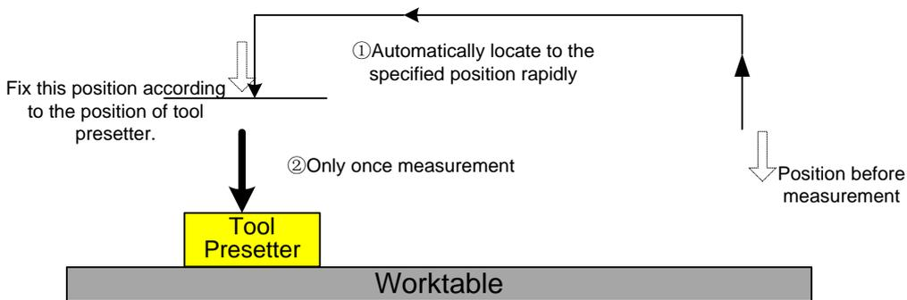
Fig. 3-27 The Process of Fixed Measurement with Encoder Feedback Function
