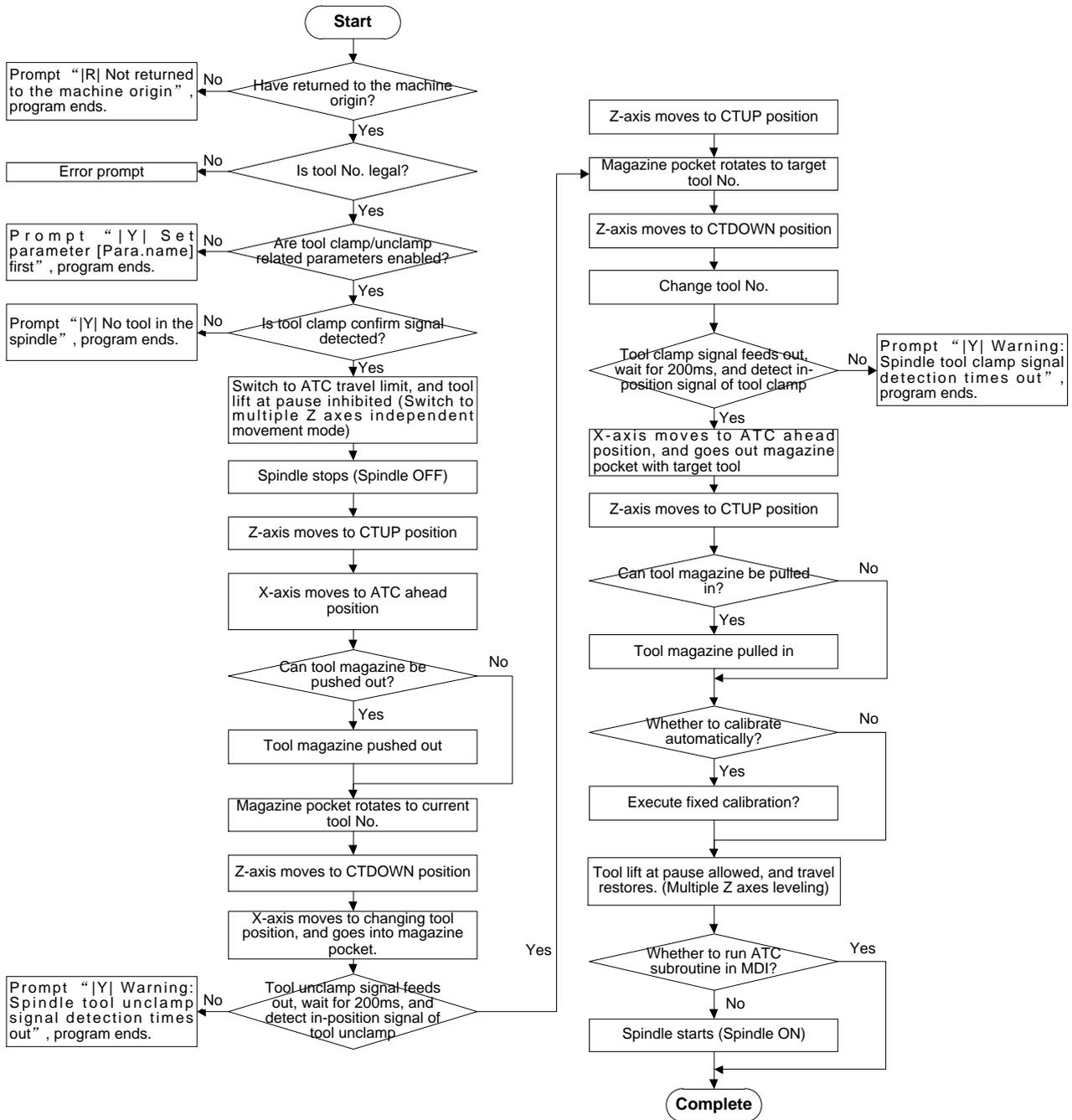
Fig. 3-101 Process of Auto Tool Change for A Circular Tool Magazine
