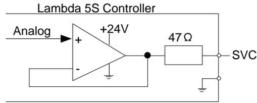
Fig. 2-5 Analog output signal circuit
