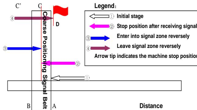
Fig. 3-12 Sketch Map of Coarse Positioning (Stopping within the Signal Belt after Receiving Coarse Positioning Signal)
