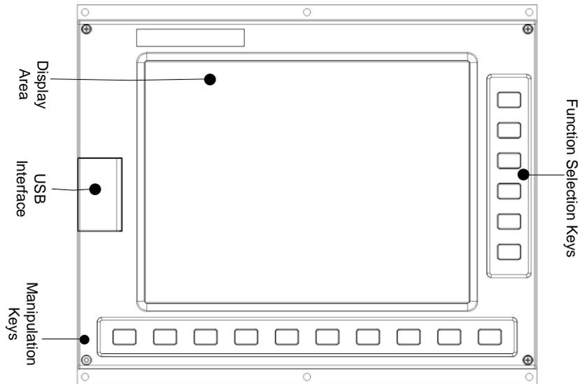
Fig. 1-3 Front view of NK300CX host
