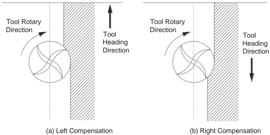
Fig. 3-53 Direction of Tool Compensation (A: Left Compensation; B: Right Compensation)
