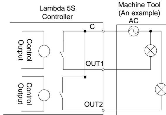
Fig. 2-2 Connection of relay output and contactor
