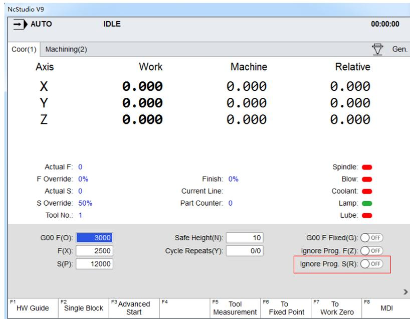
Fig. 3-21 Spindle Speed Setting
