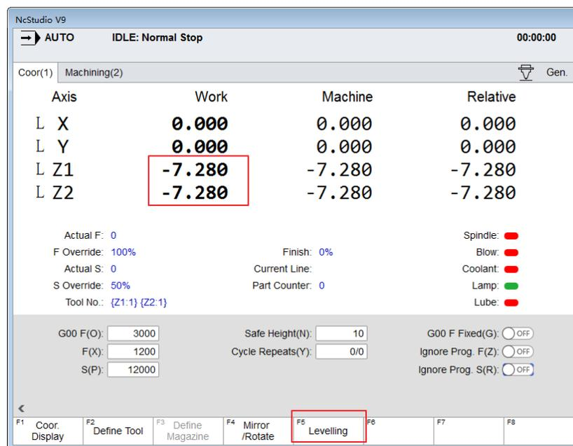
Fig. 4-2 Auto leveling Z axes
