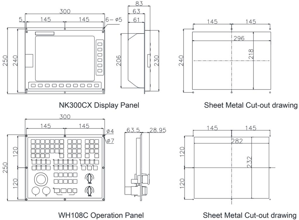
Fig. 1-16 Dimensional drawing of NK300CX-V
