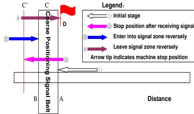
Fig. 3-13 Sketch Map of Coarse Positioning (Stopping Out of the Signal Belt after Receiving Coarse Positioning Signal)
