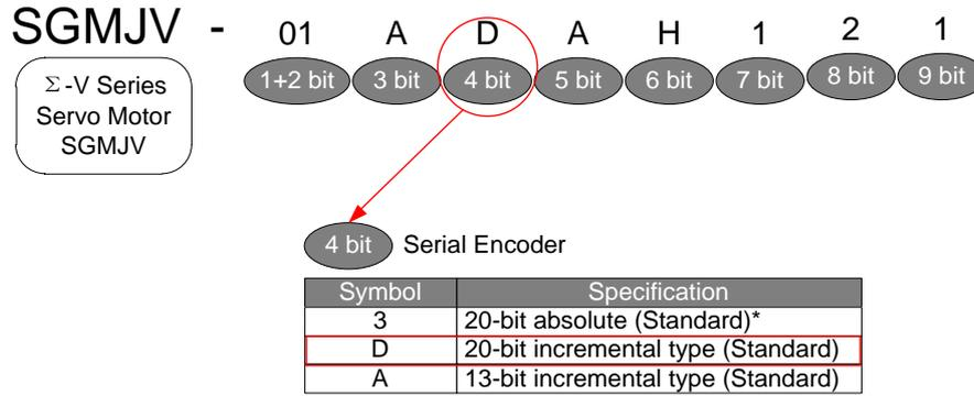
Fig. 3-18 Example of SGMJV motor nameplate
