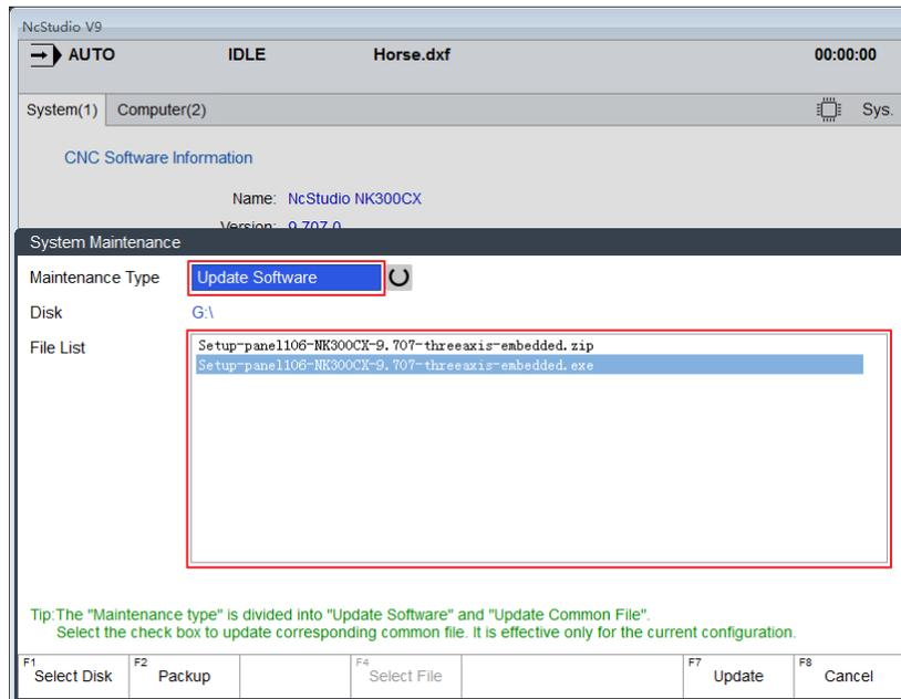
Fig. 5-11 System Maintenance- Upgrade Software
