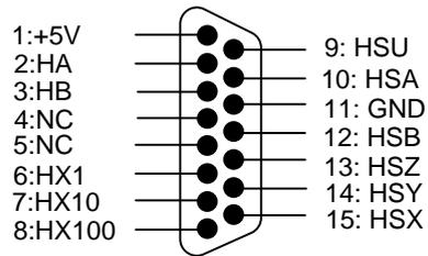
Fig. 2-8 Handwheel interface definition
