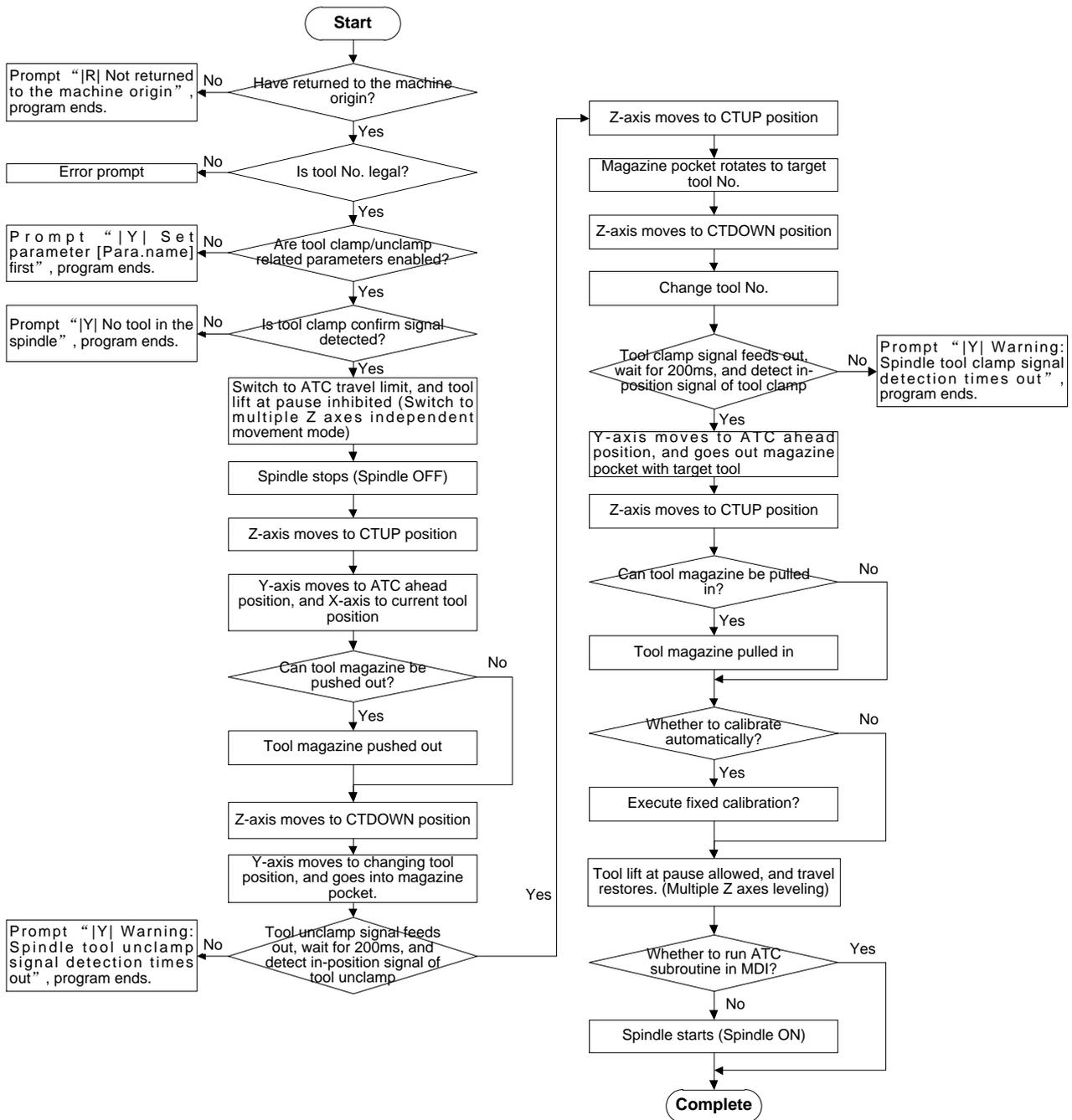
Fig. 3-102 Process of Auto Tool Change for A Servo Tool Magazine
