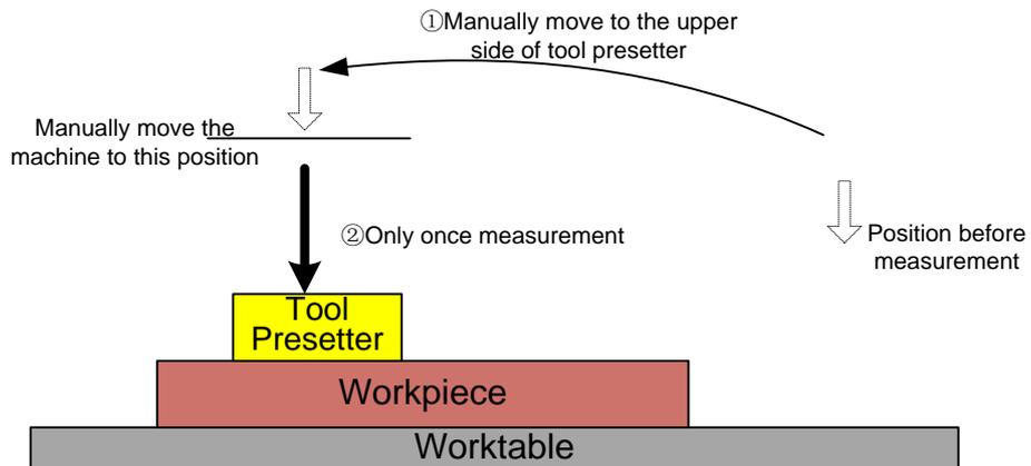
Fig. 3-31 The Process of Mobile Calibration with Encoder Feedback Function
