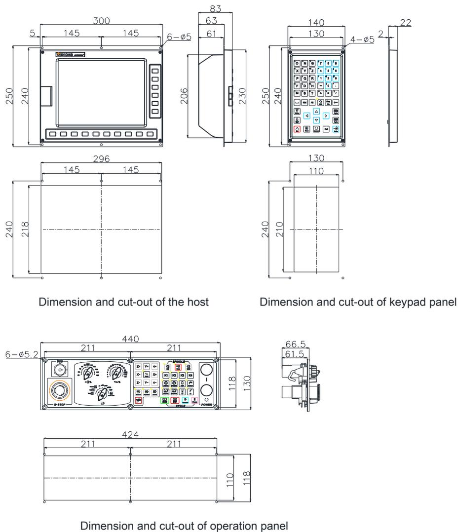
Fig. 1-15 Dimensional drawing of NK300CX-H
