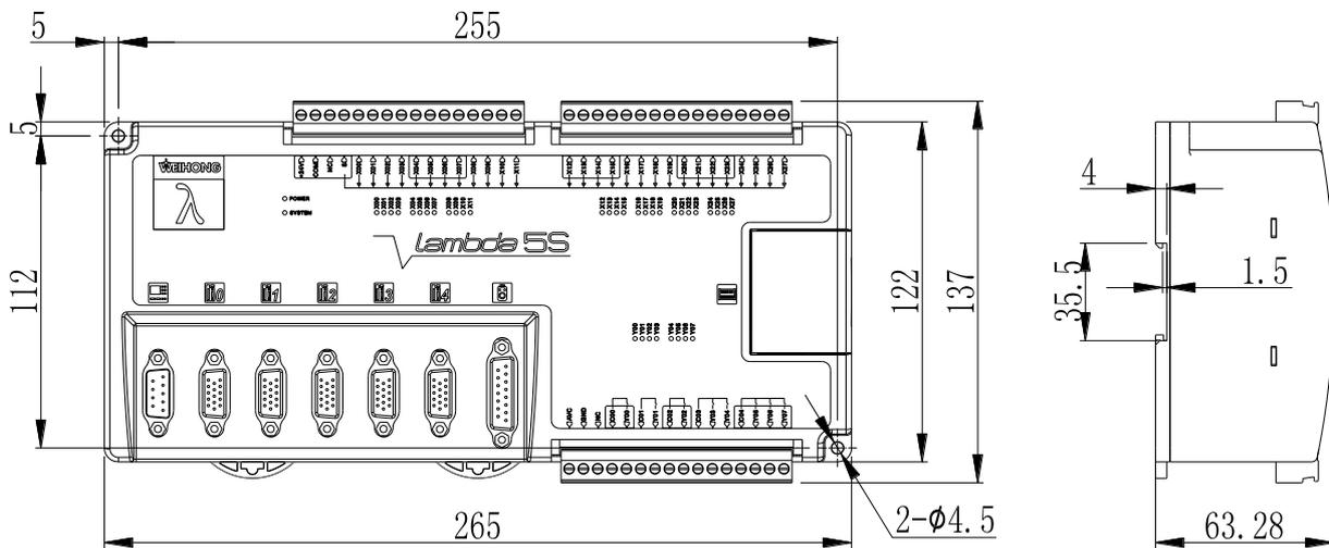
Fig. 1-17 Dimensional drawing of Lambda 5S controller
