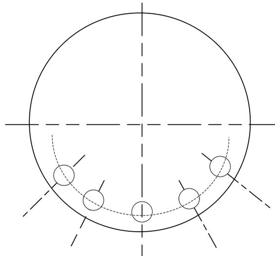
Fig. 3-100 An Example of Circular Tool Magazine
