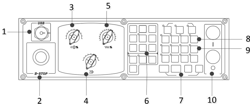
Fig. 1-5 Front view of WH106C operation panel
