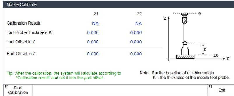
Fig. 4-4 Mobile calibration dialog box of multi-Z software
