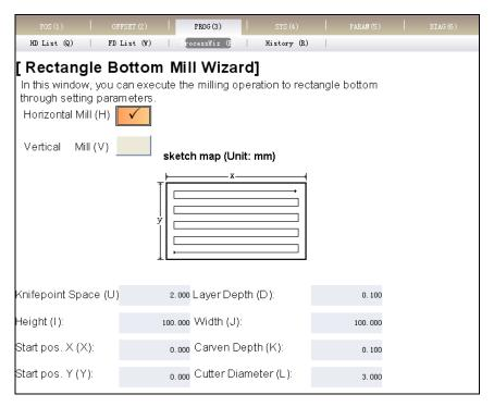
Fig. 5-41 Rectangular bottom milling function screen
