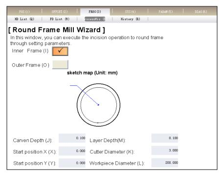
Fig. 5-40 Circular frame milling function screen
