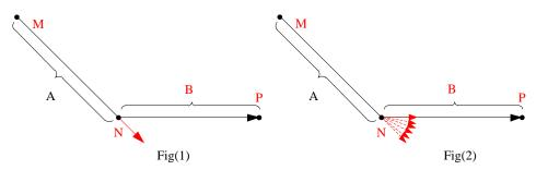
Turning Process: lift and rotate the tool at point N to the direction the tangential direction of the next part of the path and start cutting. The dotted arrow in Fig(2) represents the lifting and turning process at point N. the final direction is NP direction.
