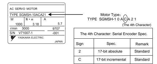
Fig. 3-2 Name plate of servo motor-encoder resolution
