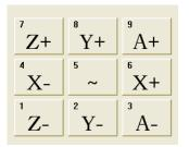
The screenshot of axis buttons is shown on the left. The number on the upper left of represents the shortcut numeric key. "~" button is the high speed button, and it has to be used along with other axis buttons.
