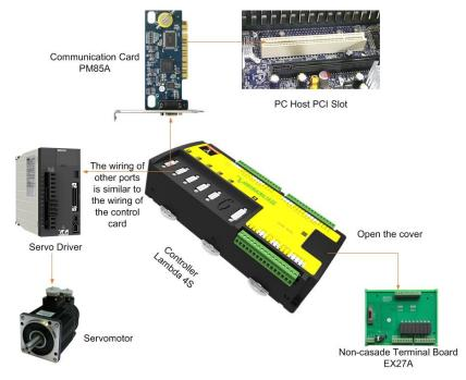
Fig. 1-1 Overall Wiring Diagram
