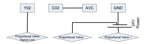
Fig. 5-2 The Wiring between Proportional Electromagnetic Valve and Port Y02
