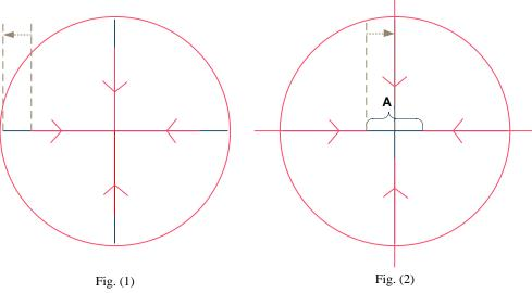
As shown in Fig. (1), the side offset exists and its value is negative, while the fore-and-aft eccentricity does not exist.
