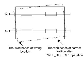
Fig. 4-4 The Diagram of X Axis Origin Detection
