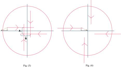
As shown in Fig. (5), both the side offset and foreand-aft eccentricity exist, and their values are both negative. The value of fore-and-aft eccentricity equals the length of line segment A. The value of the side offset equals the length of line segment B minus the length of line segment A.
