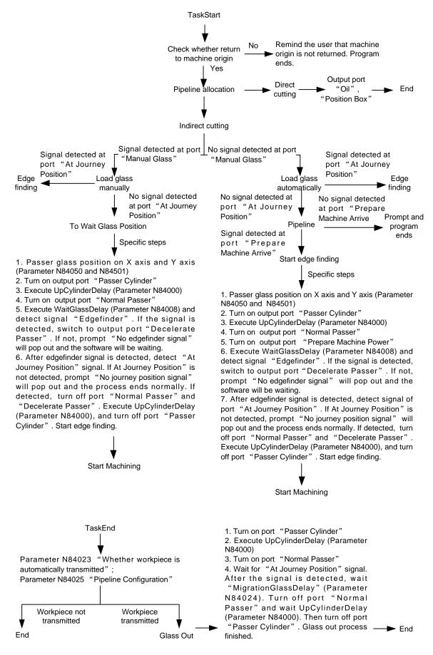
Fig. 4-19 Diagram of Assembly Line
