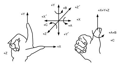
Fig. 3-1 Right-hand Rule Coordinate System
