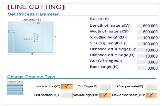
Fig. 4-14 Interface Process Wizard-Line Cutting
