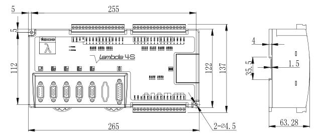
Fig. 6-1 Dimension Drawing for Lambda 4S Controller
