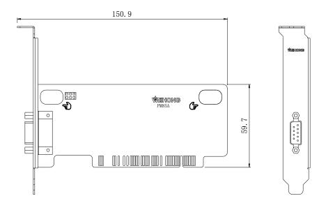
Fig. 6-3 Dimension Drawing for PM85A
