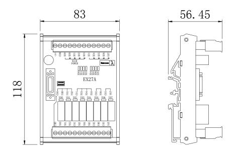
Fig. 6-2 Dimension Drawing for EX27A
