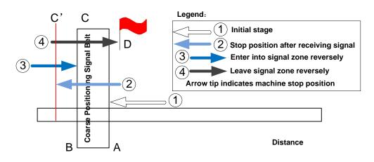
Fig. 5-2 Sketch mao of coarse positioning (stopping out of the signal belt after receiving REF. point signal)
