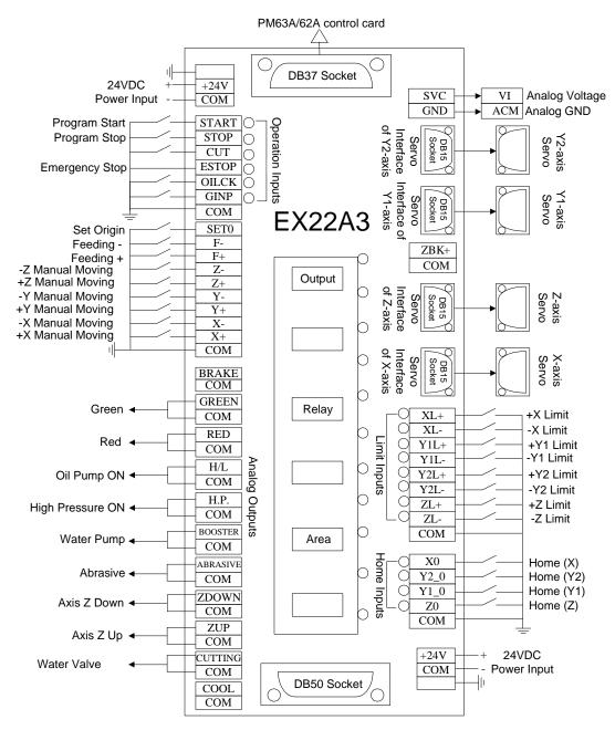
Fig. 2-5 Wiring diagram of terminal board EX22A3---for double Y axes waterjet cutting system
