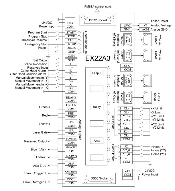
Fig. 2-7 Wiring diagram of terminal board EX22A3---for double Y axes configuration of laser cutting system
