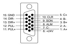
Fig. 2-15 Definition of driver interface
