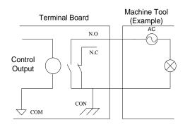
Fig. 2-11 Connection of relay output with a contactor
