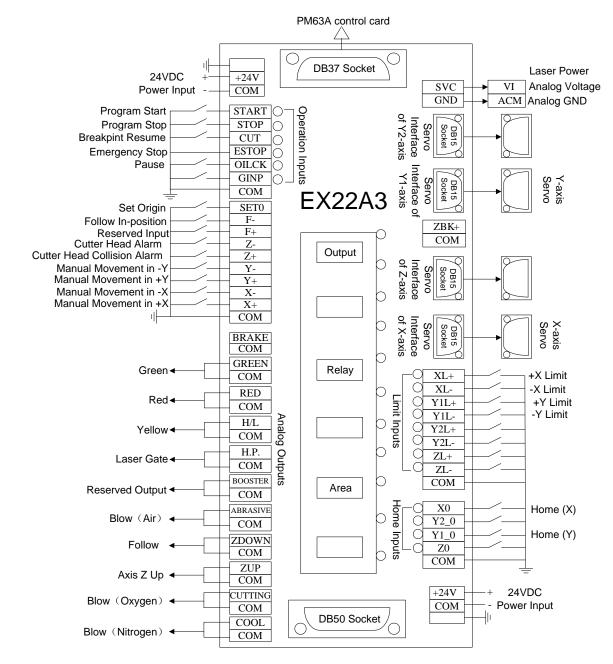
Fig. 2-6 Wiring diagram of terminal board EX22A3---for standard configuration of laser cutting system
