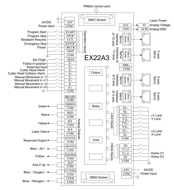
Fig. 2-8 Wiring diagram of terminal board EX22A3---for turntable configuration of laser cutting system
