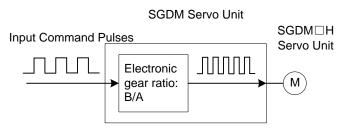
Fig. 5-8 Schematic function of "Electronic Gear Ratio"
