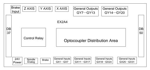
Fig. 1-3 Structure drawing of terminal board EX2A4
