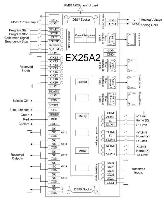
Fig. 2-1 Wiring diagram of terminal board EX25A2---for engraving and milling system
