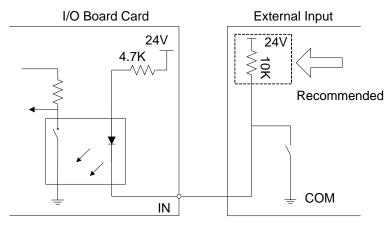
Fig. 2-10 Binary input connecting with a photoelectric switch or a proximity switch **2.2.2. Relay Output Signal**
