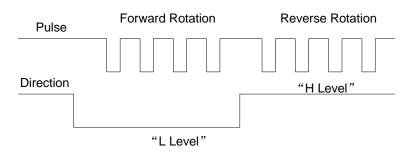
Fig. 2-12 Output type of pulse command The output form of differential signal is shown in Fig. 2-13.
