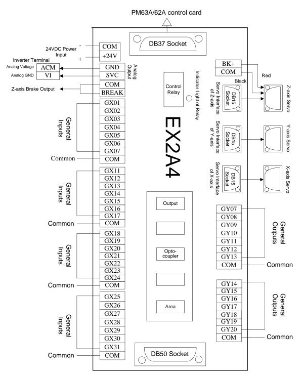
Fig. 2-3 Wiring diagram of terminal board EX2A4
