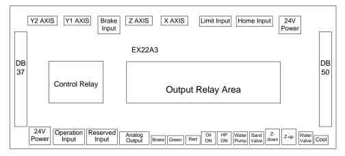
Fig. 1-5 Structure drawing of terminal board EX22A3
