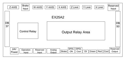
Fig. 1-2 Structure drawing of terminal board EX25A2
