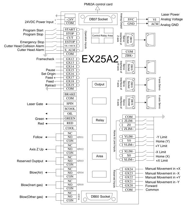
Fig. 2-2 Wiring diagram of terminal board EX25A2---for laser cutting system
