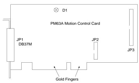
Fig. 1-1 Structural drawing of PM63Acontrol card
