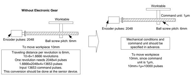
Fig. 5-7 Schematic conversion of electric gear ratio 5.2.3. Computing Method of Electronic Gear Ratio
