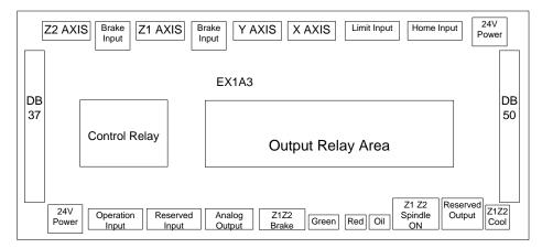
Fig. 1-4 Structure drawing of terminal board EX1A3
