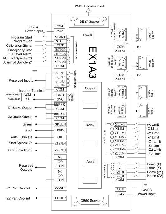
Fig. 2-4 Wiring diagram of terminal board EX1A3
