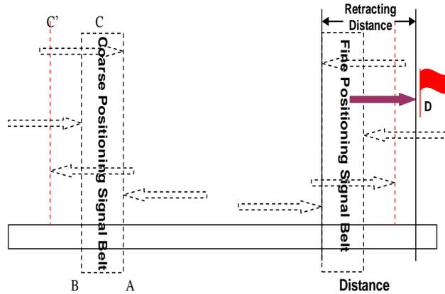
Fig. 3-15 Retracting Stage
