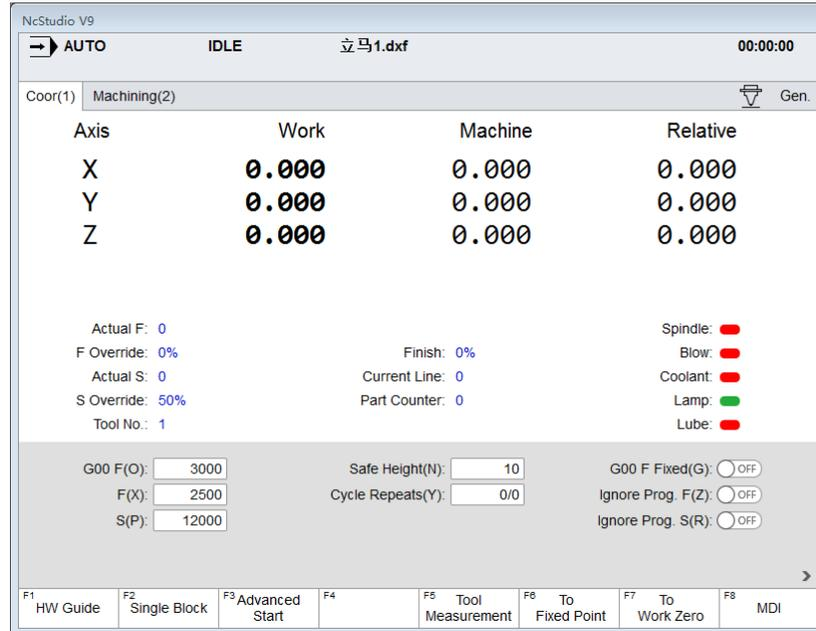
Fig. 1-21 Example of main interface of standard type of 3 axes software
