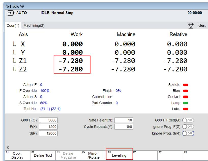
Fig. 4-2 Auto leveling Z axes
