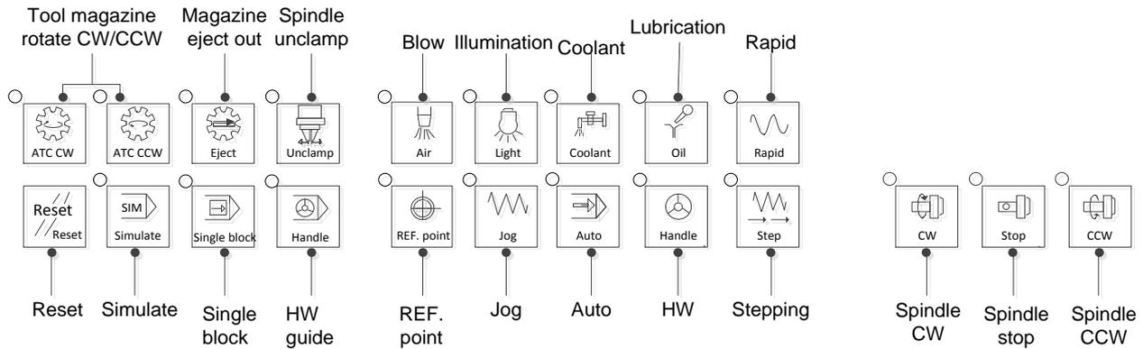
Fig. 1-13 Auxiliary function keys and mode selection keys
