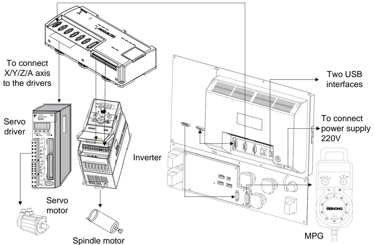
Fig. 1-19 Overall connection diagram of NK300CX-H
