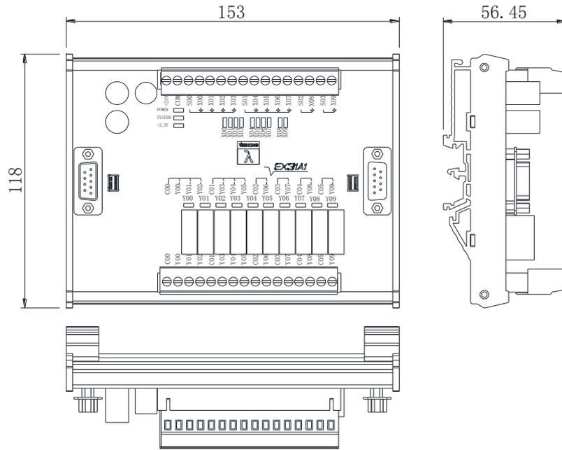
Fig. 1-18 Dimensional drawing of EX31A1
