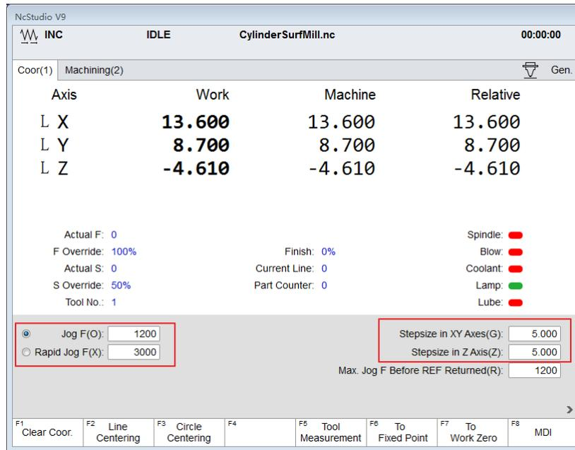
Fig. 3-46 Setting of Jog Speed and Rapid Jog Speed
