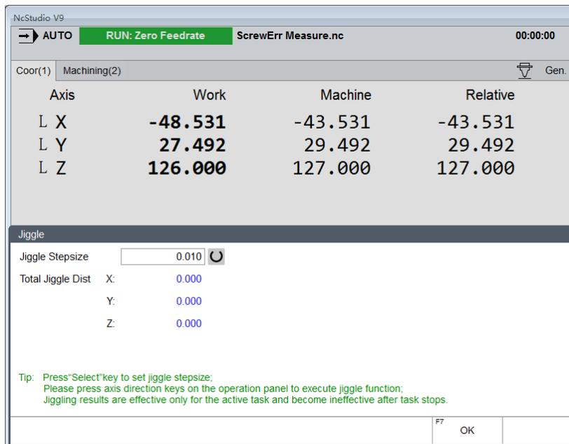
Fig. 3-91 Jiggle Setup
