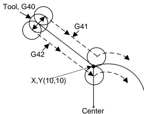
Fig. 3-54 Schematic Diagram of Tool Compensation Machining
