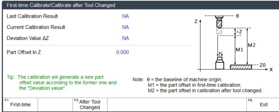
Fig. 3-32 Dialog Box "First Calibration/Calibration after Tool Changed"
