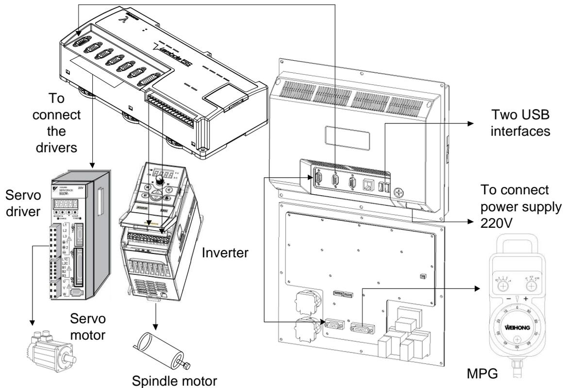
Fig. 1-20 Overall connection diagram of NK300CX-V
