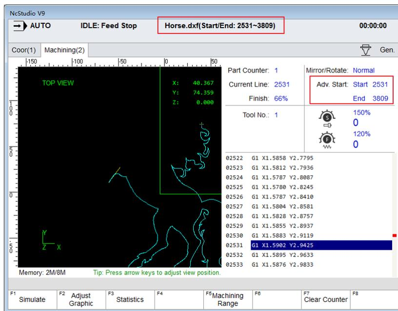
Fig. 3-93 View the Start and End Line Number of Advanced Start
