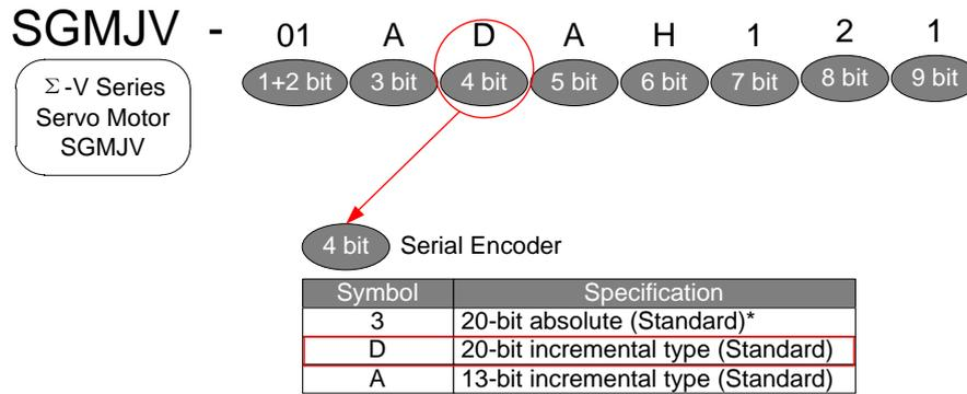
Fig. 3-18 Example of SGMJV motor nameplate
