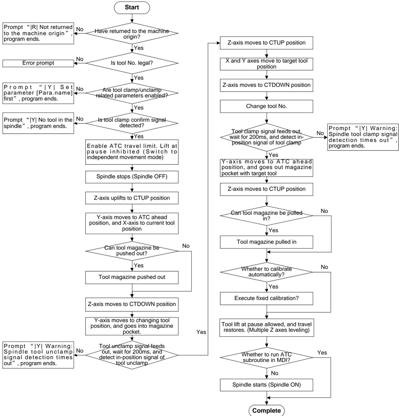
Fig. 3-99 Process of Auto Tool Change for A Linear Tool Magazine
