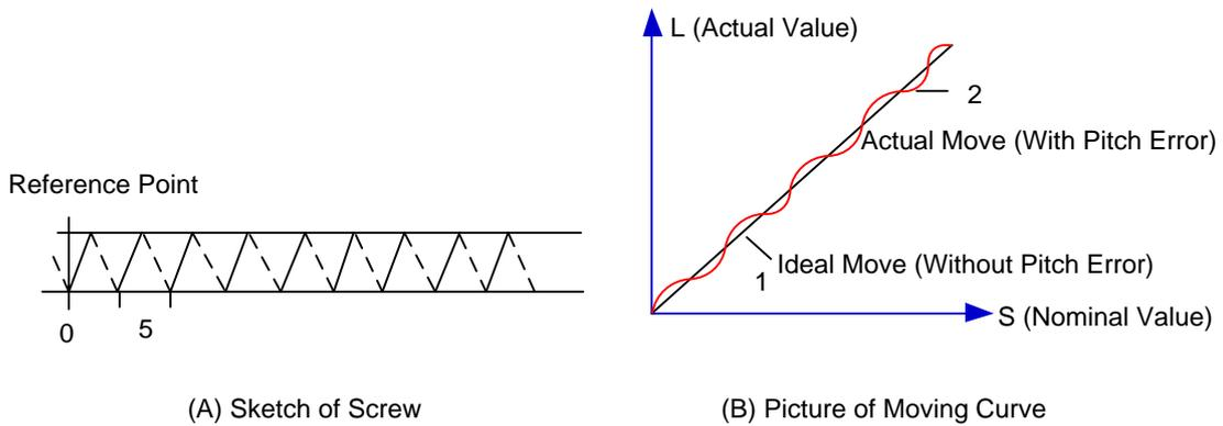
Fig. 3-57 Analysis of Pitch Error
