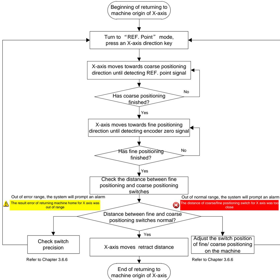
Fig. 3-6 The Process of Returning to Machine Origin (X-axis)
