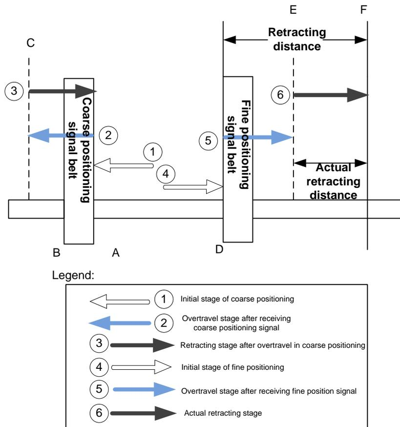
Fig. 3-16 The Process of Returning to Machine Origin
