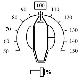
Fig. 3-22 Spindle Override Knob
