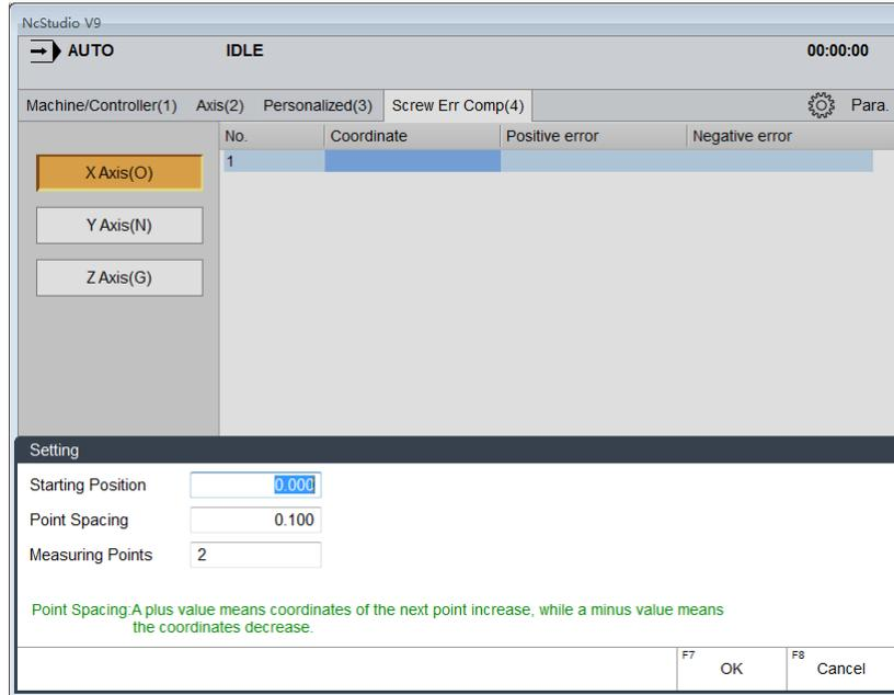
Fig. 3-61 Setting-[Screw Err Comp(4)]
