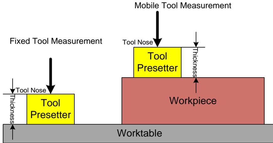
Fig. 3-24 Sketch Map of Using A Tool Presetter
