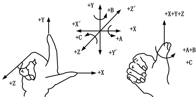
Fig. 3-4 Standard Coordinate System of Right-hand Rule
