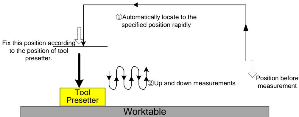
Fig. 3-26 The Process of Fixed Calibration without Encoder Feedback Function
