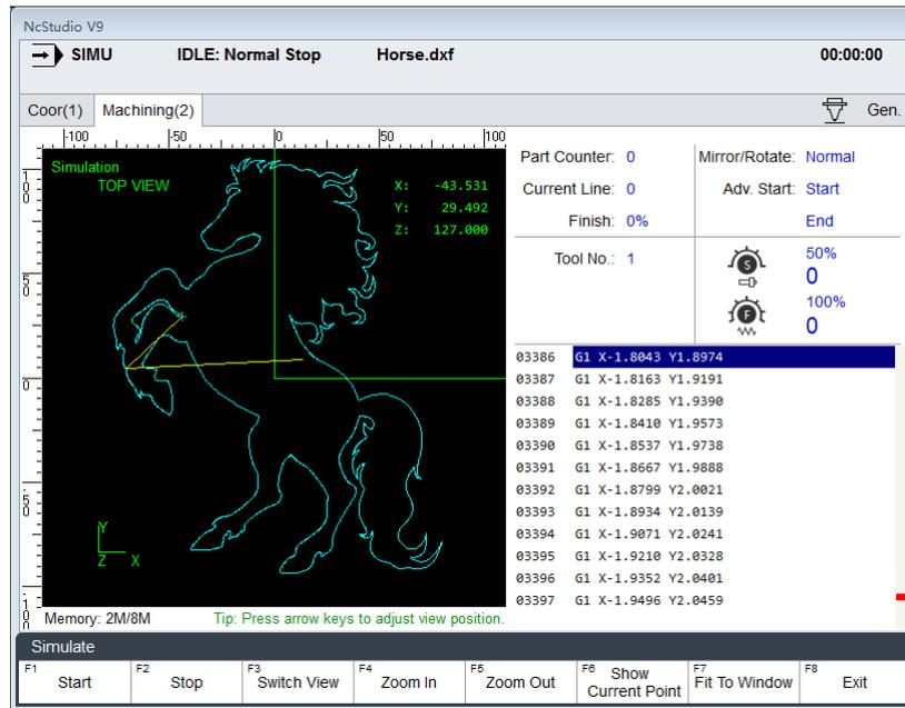
Fig. 3-47 Simulation and Track Window
