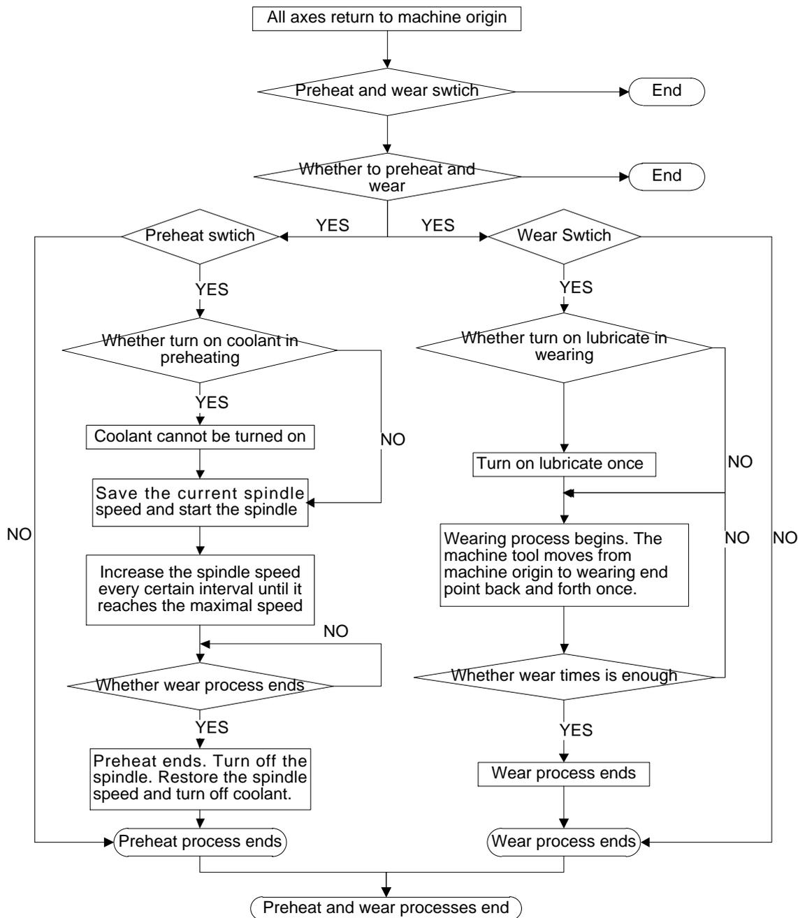
Fig. 3-20 Flow Chart of Preheat and Wear Function
