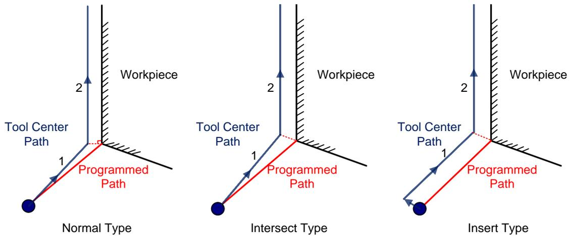
Fig. 3-52 Type to Establish Tool Compensation
