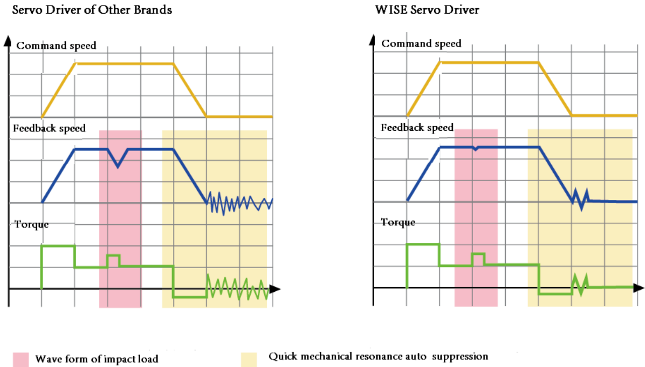
Fig. 1-2 Comparison between counterparts and WISE servo driver
