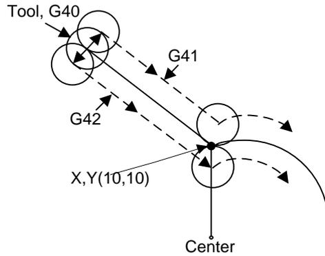
Fig. 3-45 Schematic Diagram of Tool Compensation Processing
