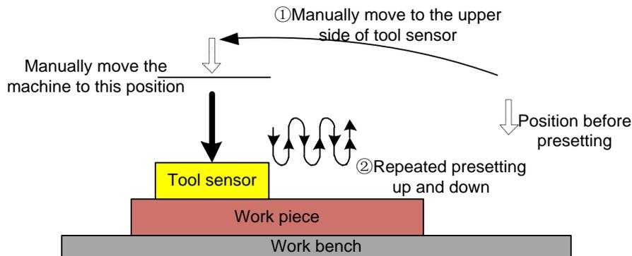
Fig. 3-24 The Process of Floating Presetting
