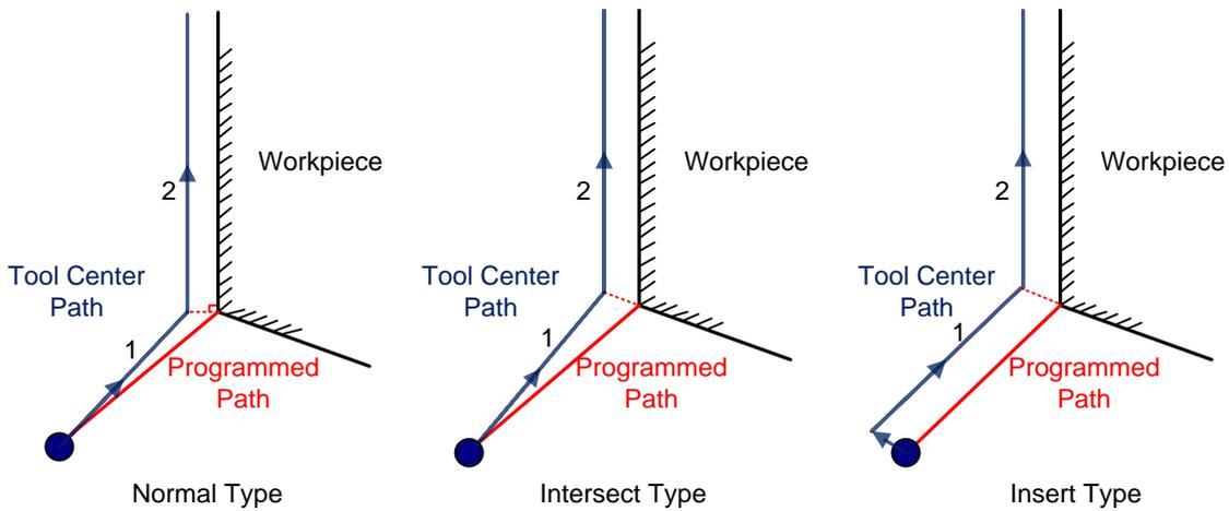
Fig. 3-43 Types of Enabling Tool Compensation
