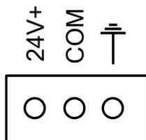
Fig. 2-7 Pins Definition of +24V Power Input Interface
