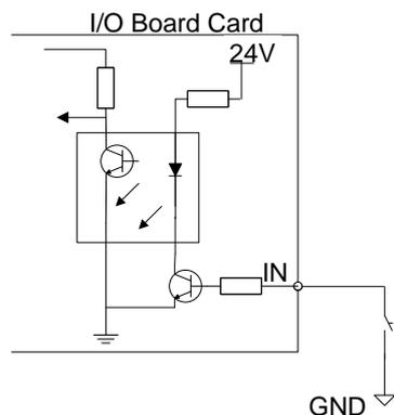
Fig. 2-1 Connection of Mechanical Switch and Binary Input
