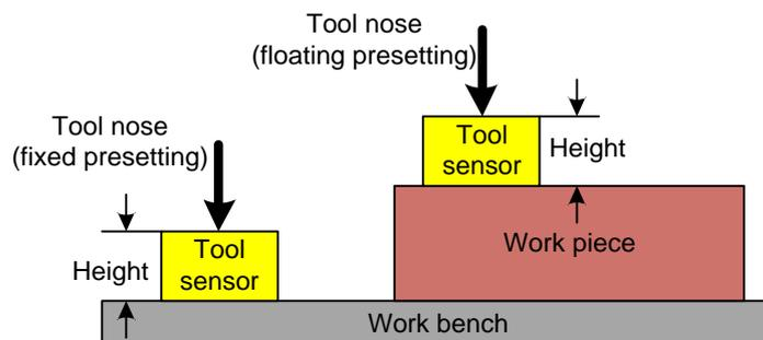
Fig. 3-22 Sketch Map of Using Tool Sensor
