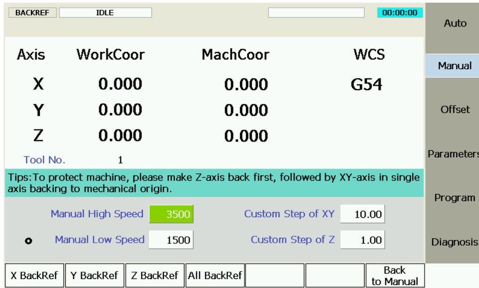
Fig. 3-13 Interface of Backing to Machine Origin
