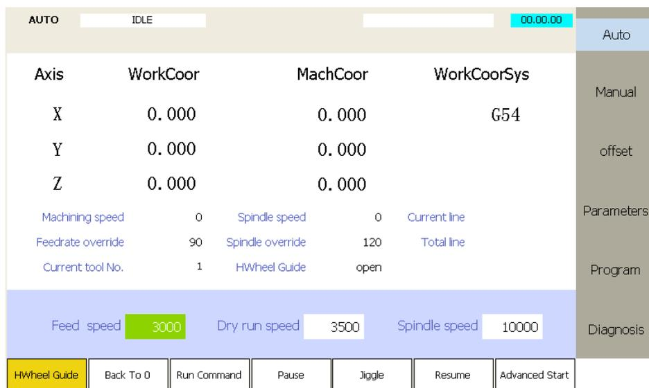
Fig. 3-59 Handwheel Guide Interface
