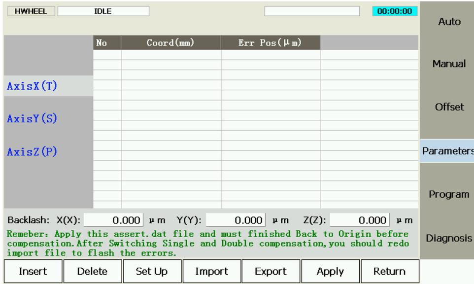
Fig. 3-39 Compensation Parameters Setting
