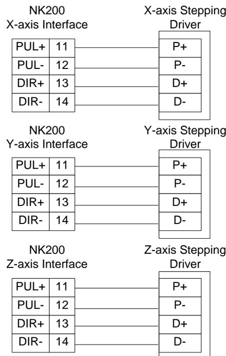
Fig. 5-1 Connection between NK200 and differential input stepping driver
