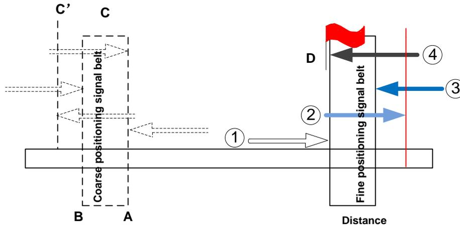
Fig. 3-11 The Process of Fine Positioning
