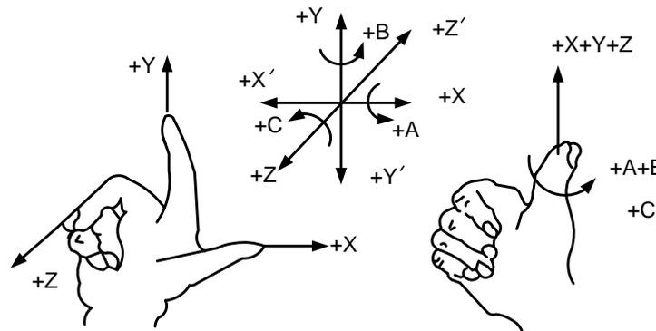
Fig. 3-6 The Coordinate System of the Right Hand Principle
