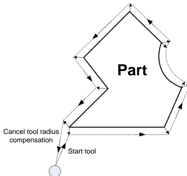
Fig. 3-42 Tool Radius Compensation Illustration
