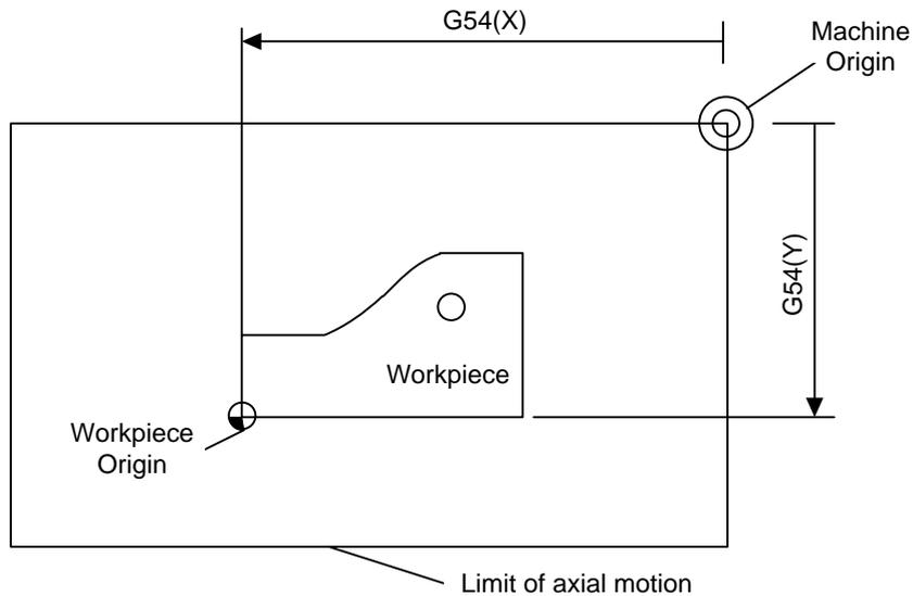
Fig. 3-29 The Relationship of Workpiece Offset and Mechanical Coordinate System
