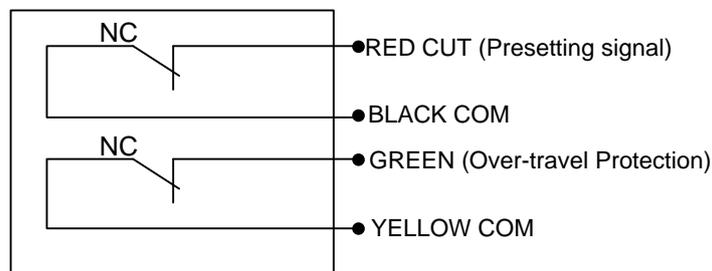
Fig. 3-21 Electrical Wiring Diagram of Tool Sensor
