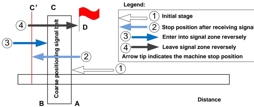
Fig. 3-10 Sketch Map of Coarse Positioning (Stopping out of the signal belt after receiving coarse positioning signal)
