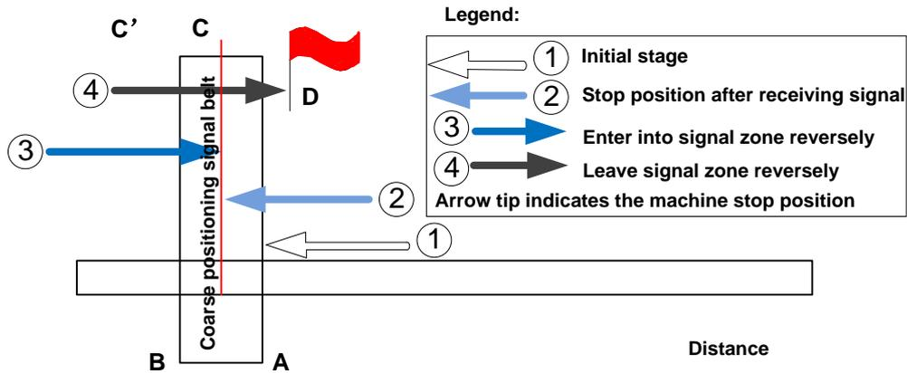
Fig. 3-9 Sketch map of coarse positioning (stopping within the signal belt after receiving coarse positioning signal)
