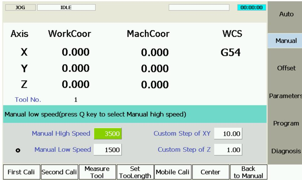
Fig. 3-23 Sub-screen of Tool Presetting
