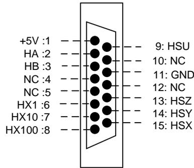
Fig. 2-11 Handwheel Interface Definition
