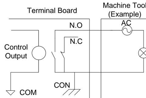
Fig. 2-5 Connection of Relay Output and Contactor
