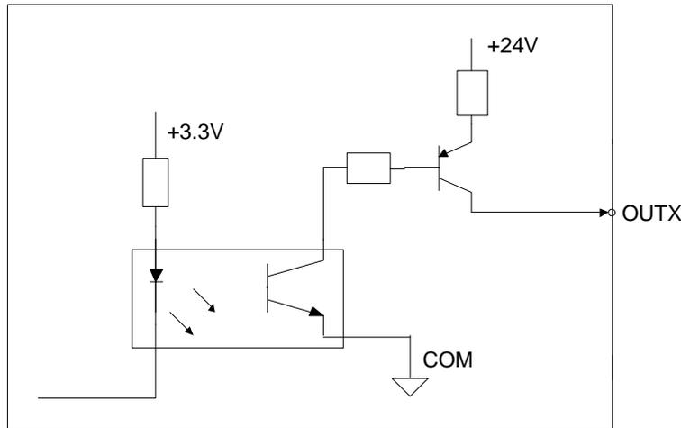
Fig. 2-3 Equivalent Circuit of Binary Output Interface
