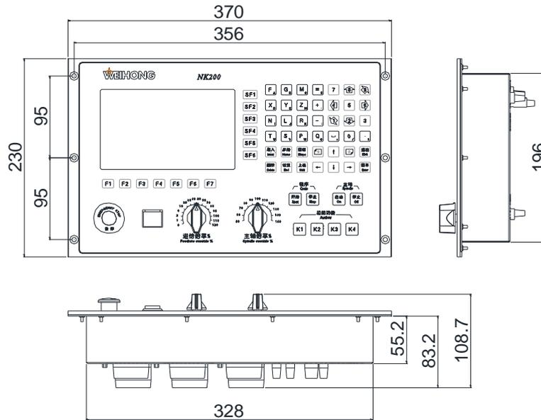
Fig. 1-4 Mounting Dimension of NK200
