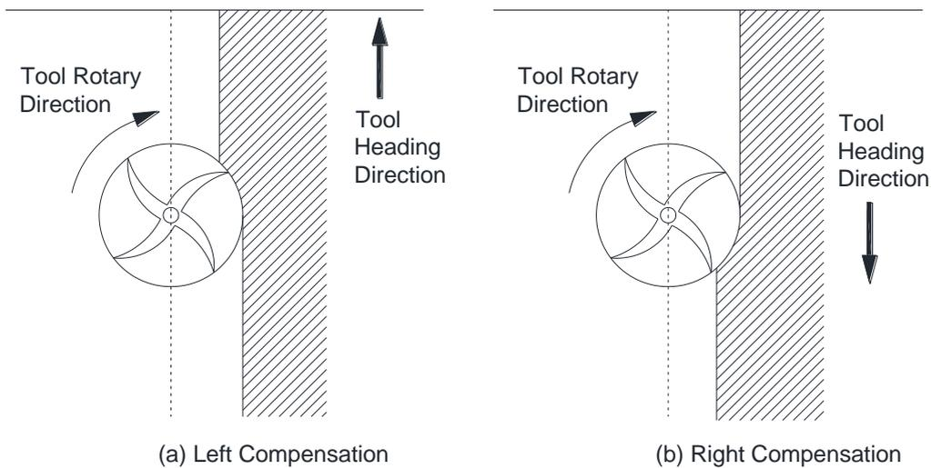
Fig. 3-44 Direction of Tool Compensation (a: Left compensation b: Right compensation)
