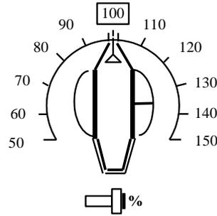
Fig. 3-17 Spindle Override Selection Switch
