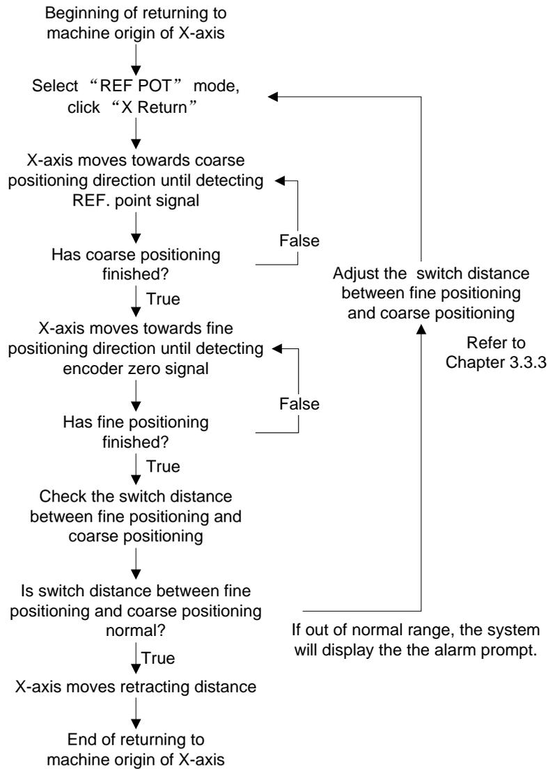
Fig. 3-8 The Process of Returning to Machine Origin (X-axis)
