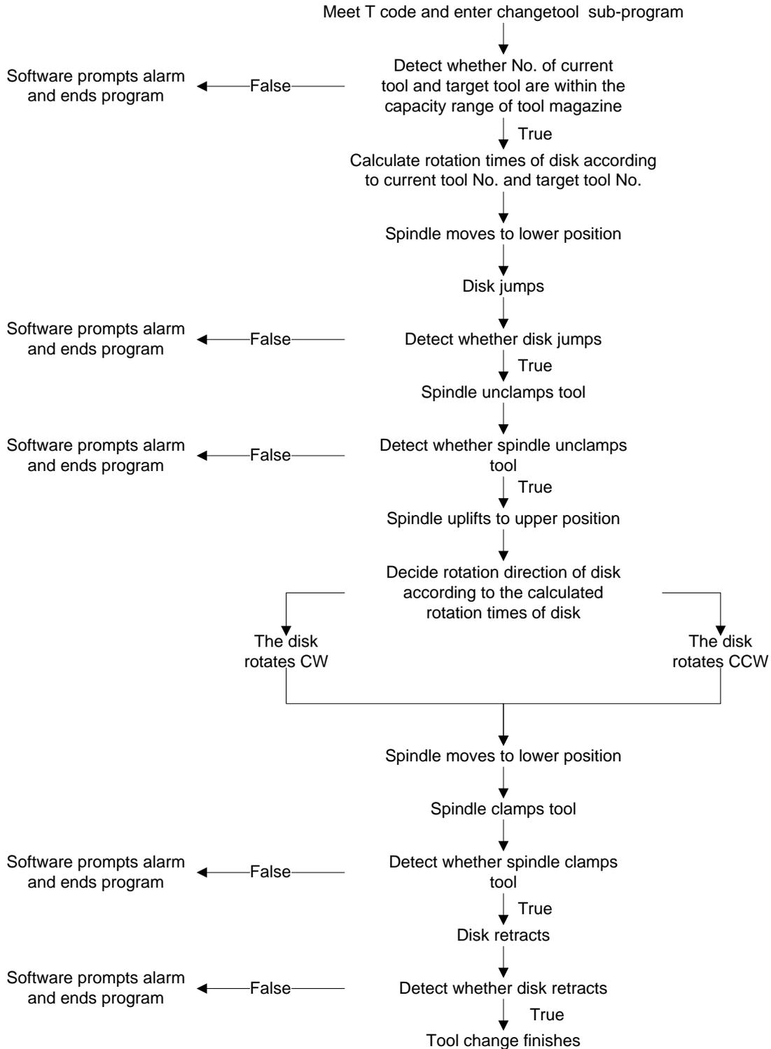
Fig. 3-72 Process of Auto Tool Change for Circular Tool Magazine
