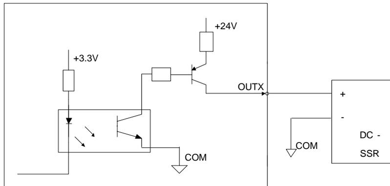
Fig. 2-4 Connection of Solid-state Relay and Binary Output
