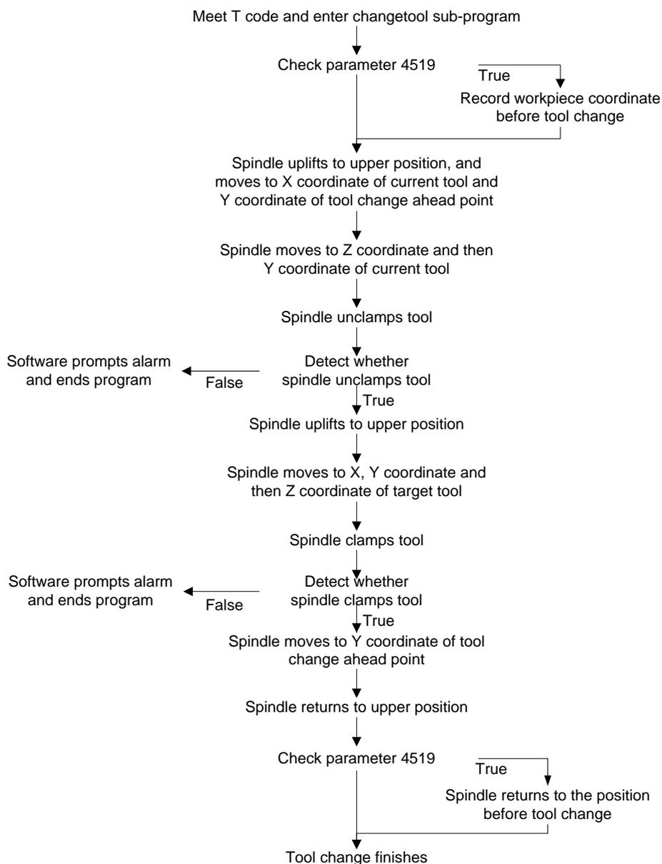
Fig. 3-71 Process of Auto Tool Change for Linear Tool Magazine
