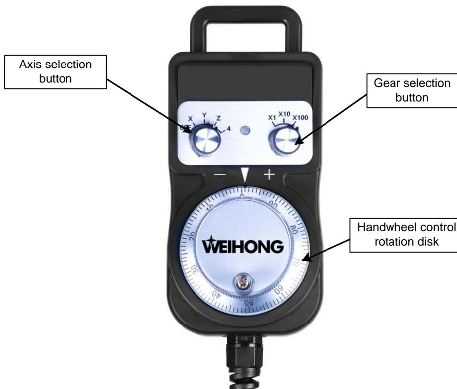
Fig. 3-58 Handwheel
