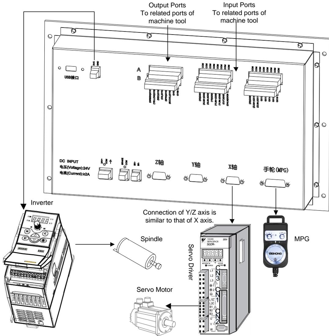
Fig. 1-6 Connection Schematic Diagram of NK200
