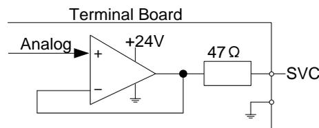
Fig. 2-6 Electric Circuit of Analog Output Signal
