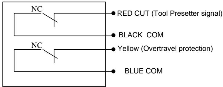
Fig. 3-26 Electrical wiring diagram of a WEIHONG tool presetter
