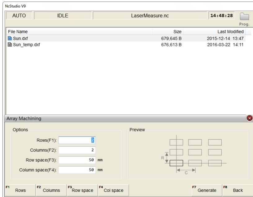
Fig. 3-83 Array machining process
