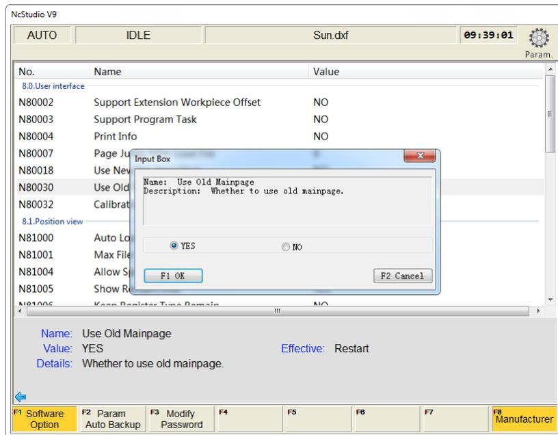
Fig. 3-4 Parameter setting for interface switchover
