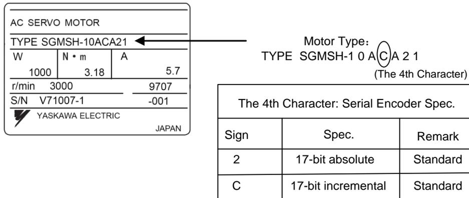
Fig. 3-8 Servo motor brand-encoder resolution
