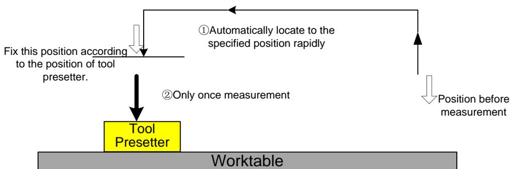
Fig. 3-33 The process of fixed measurement with encoder feedback function
