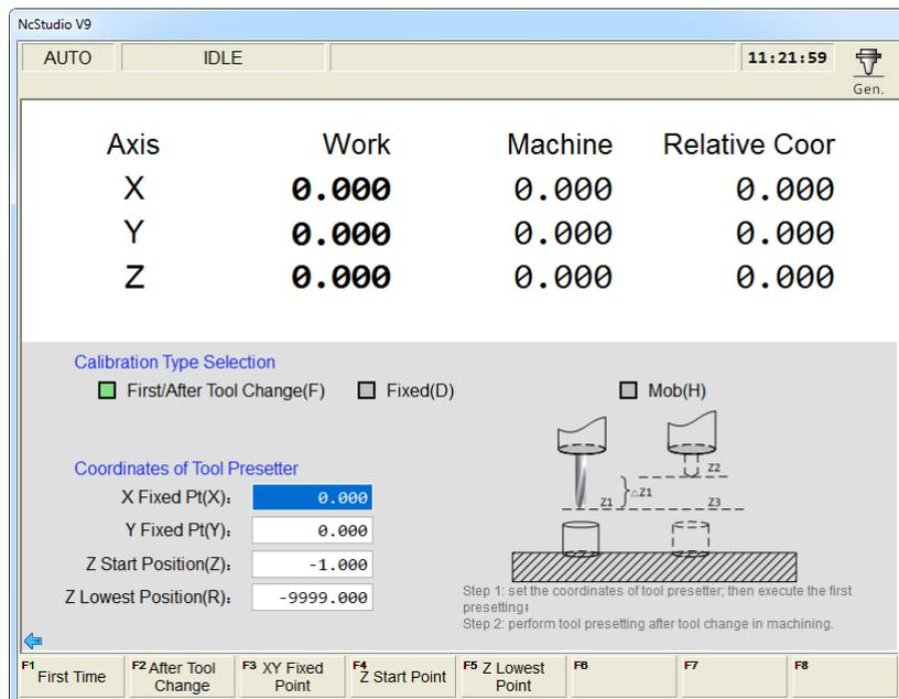
Fig. 3-29 First calibration/calibration after tool change
