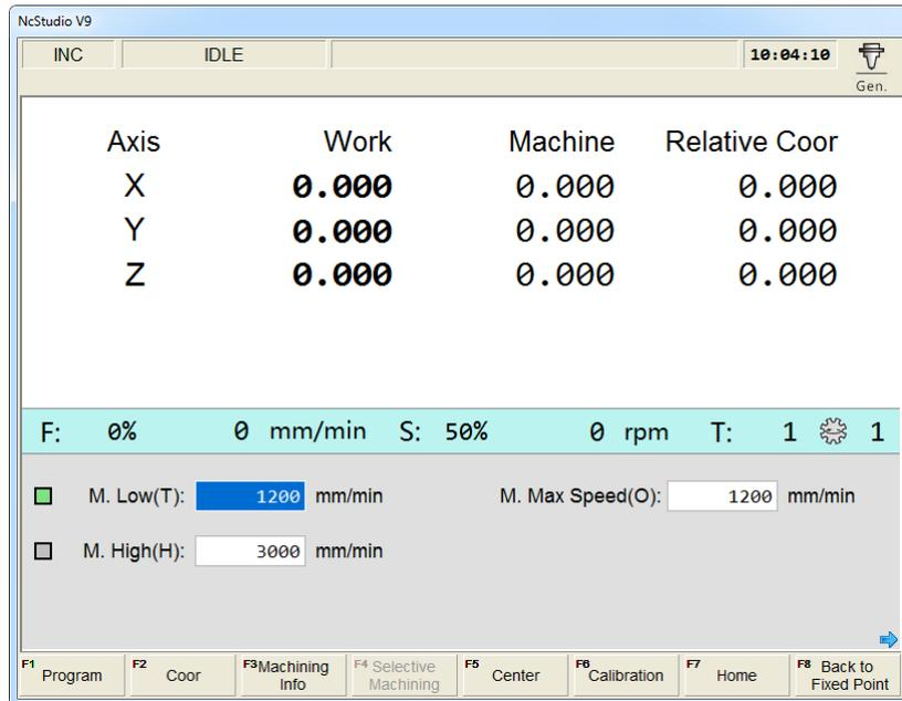
Fig. 3-57 Manual high/low speed setting in new interface
