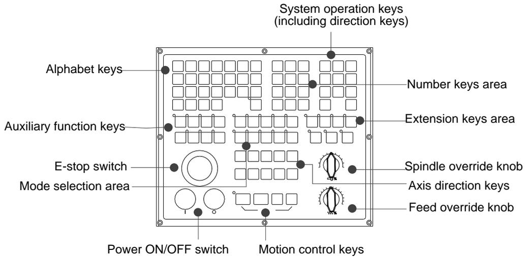
Fig. 1-14 Front view of operation panel WH108A1
