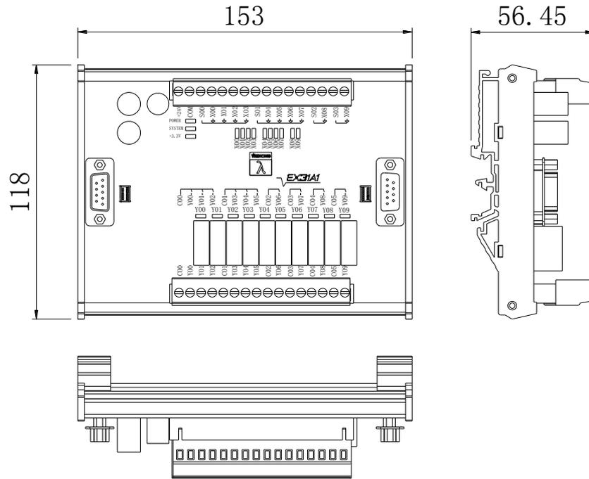
Fig. 2-9 Mounting Dimension of Terminal Board EX31A1
