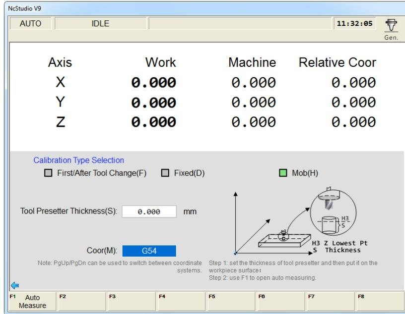
Fig. 3-36 Mobile Calibration
