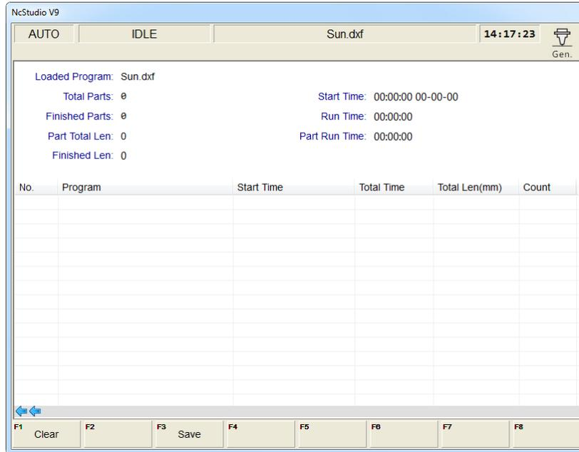
Fig. 3-61 Machining statistics window
