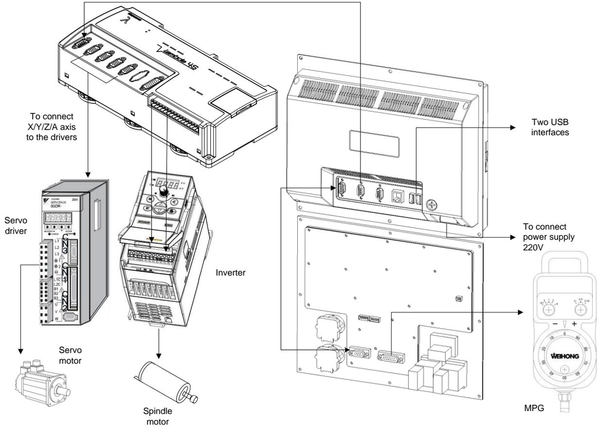
Fig. 1-18 Overall connection diagram of NK300BX-V
