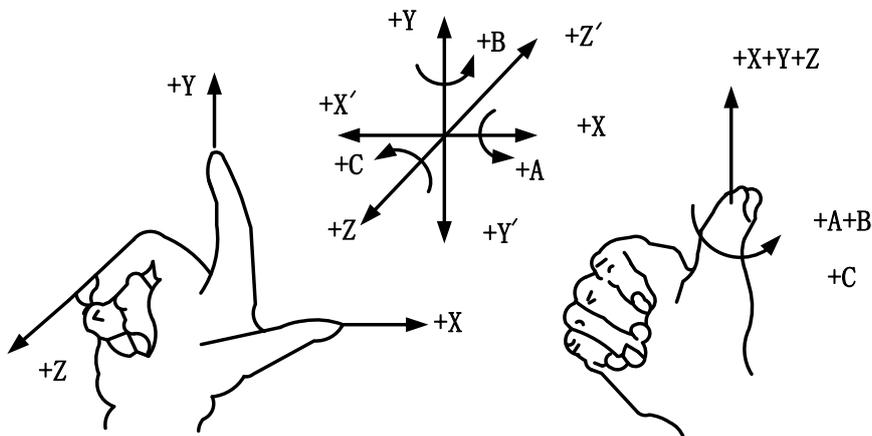
Fig. 3-7 Standard coordinate system of right-hand rule
