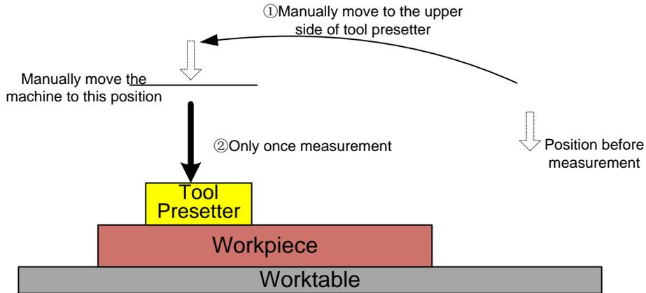
Fig. 3-38 The process of mobile calibration with encoder feedback function
