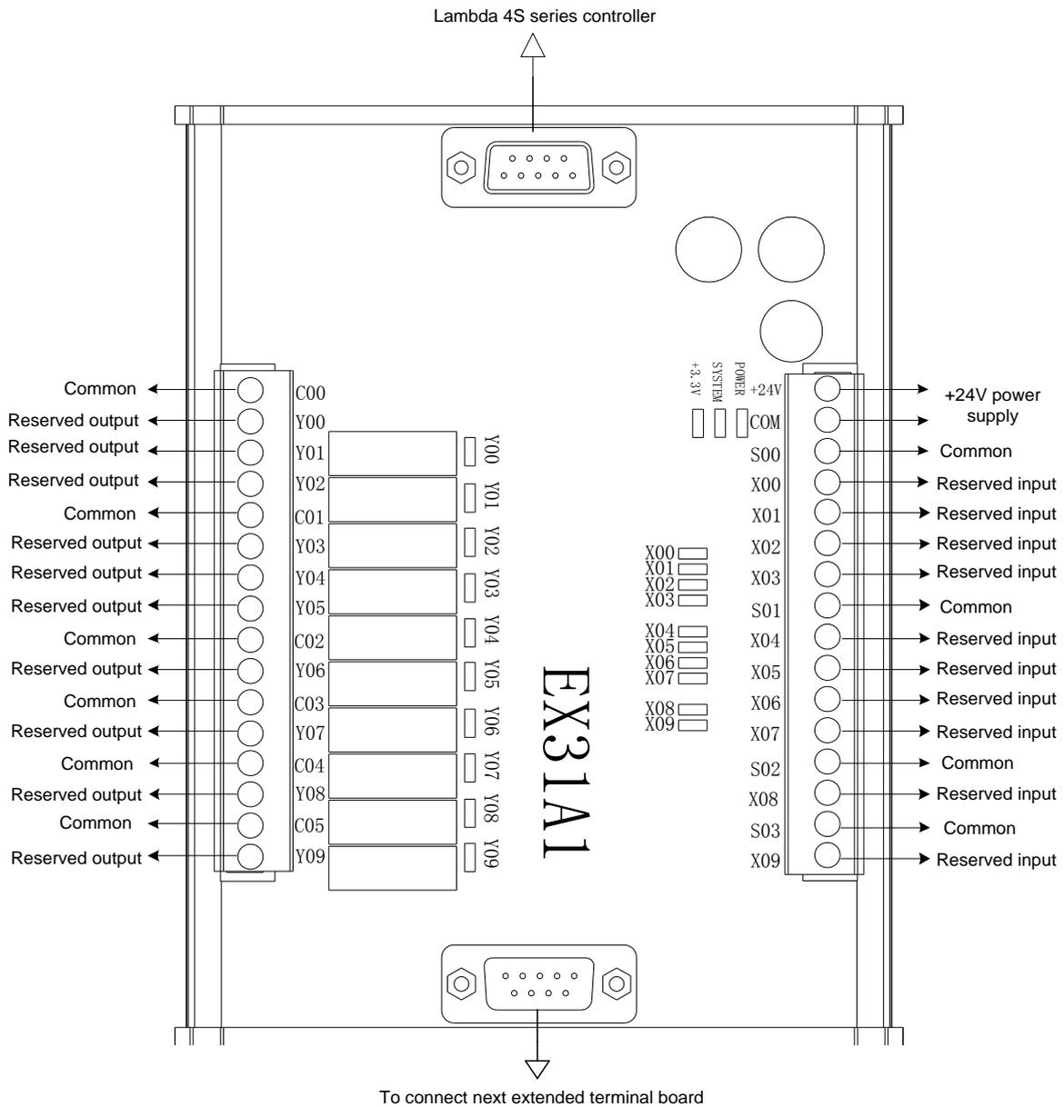
Fig. 2-10 Wiring diagram of terminal board EX31A1
