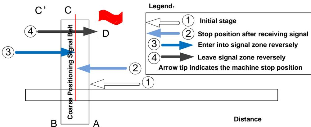
Fig. 3-17 Sketch map of coarse positioning (stopping within the signal belt after receiving coarse positioning signal)
