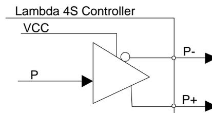
Fig. 2-4 Pulse Command Output Circuit
