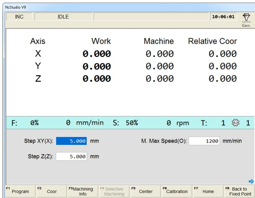
Fig. 3-58 User-defined step length setting in new interface
