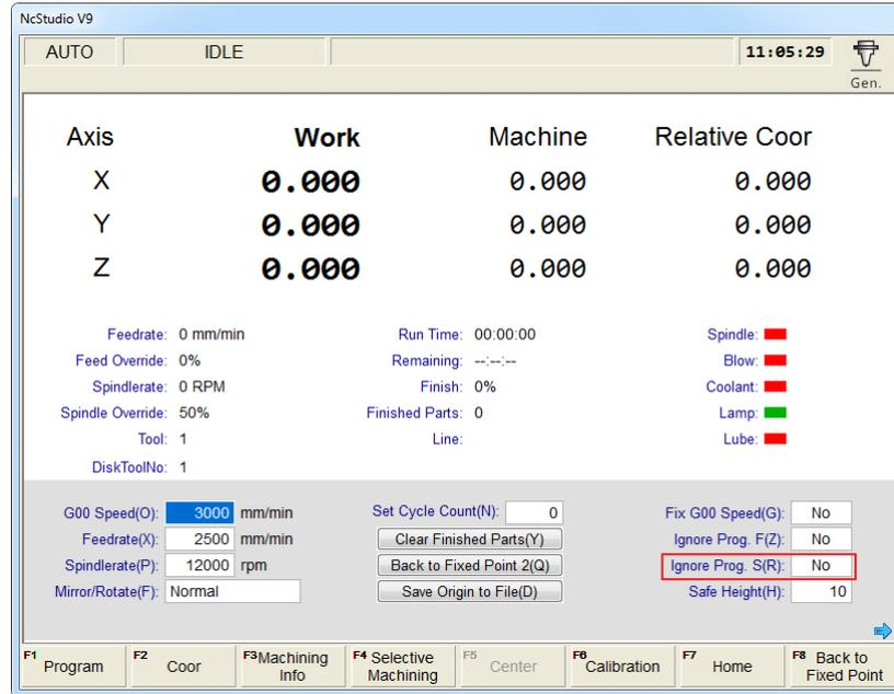
Fig. 3-23 Spindle speed setting on classic interface
