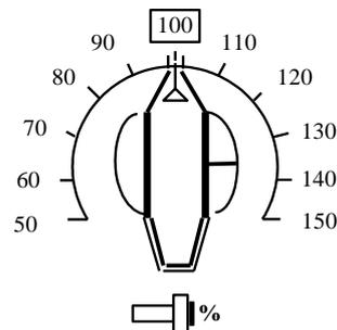
Fig. 3-25 Spindle override knob
