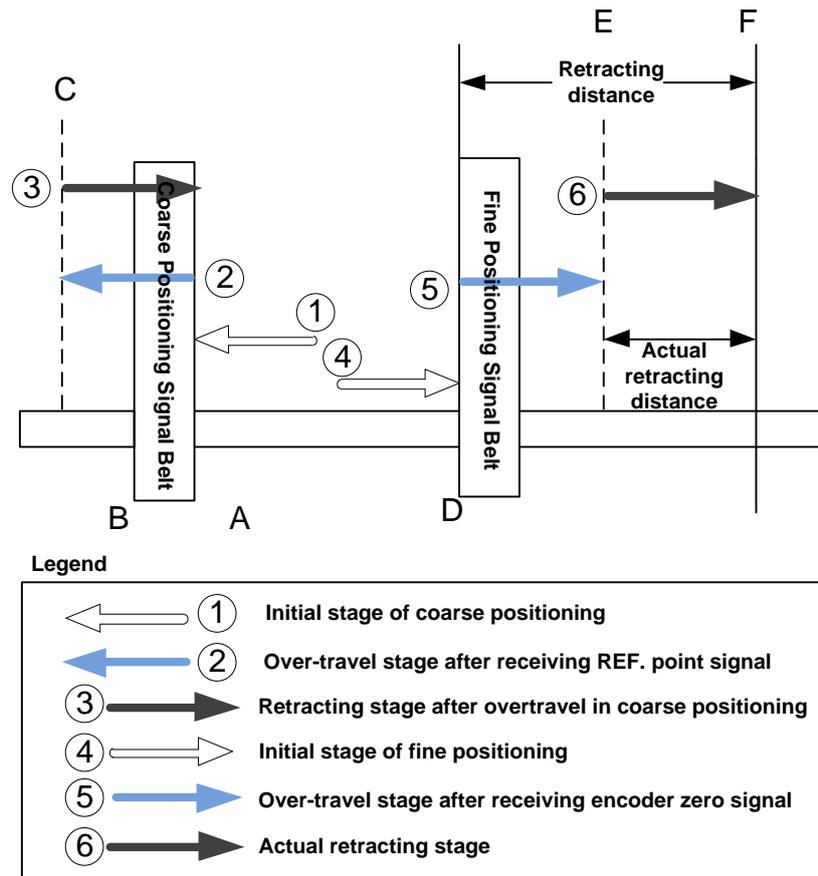
Fig. 3-21 The process of returning to machine origin
