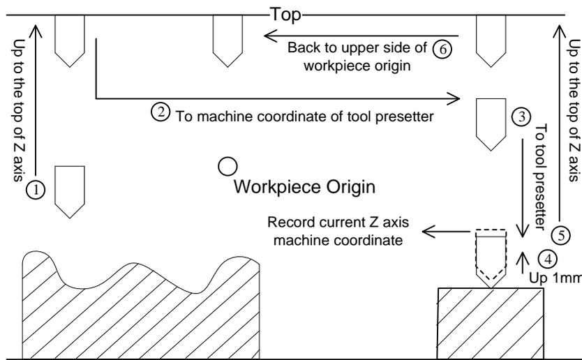
Fig. 3-30 First tool measurement
