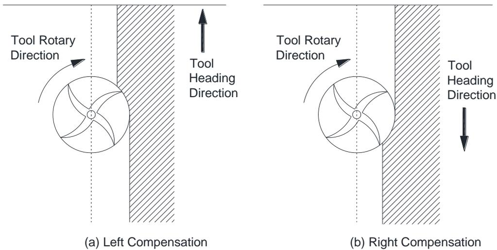
Fig. 3-65 Direction of tool compensation (a: left compensation b: right compensation)
