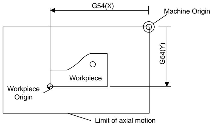
Fig. 3-39 The relationship of work offset and machine coordinate system
