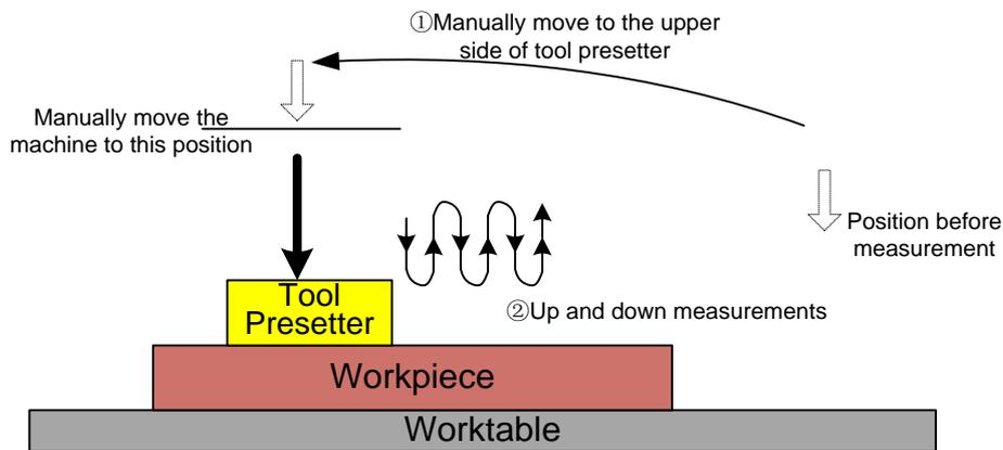
Fig. 3-37 The process of mobile calibration without encoder feedback function
