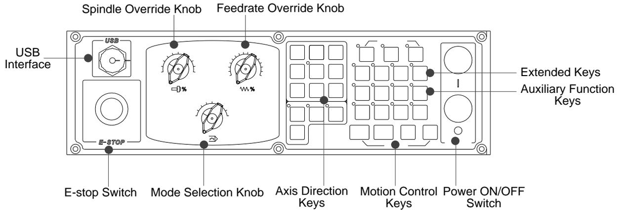
Fig. 1-7 Front view of operation panel WH106A3
