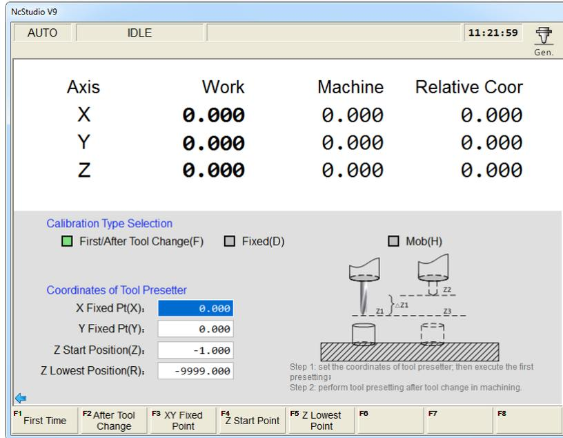
Fig. 3-28 Sub-screen of tool measurement
