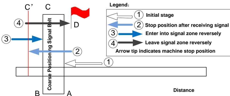
Fig. 3-18 Sketch map of coarse positioning (stopping out of the signal belt after receiving coarse positioning signal)
