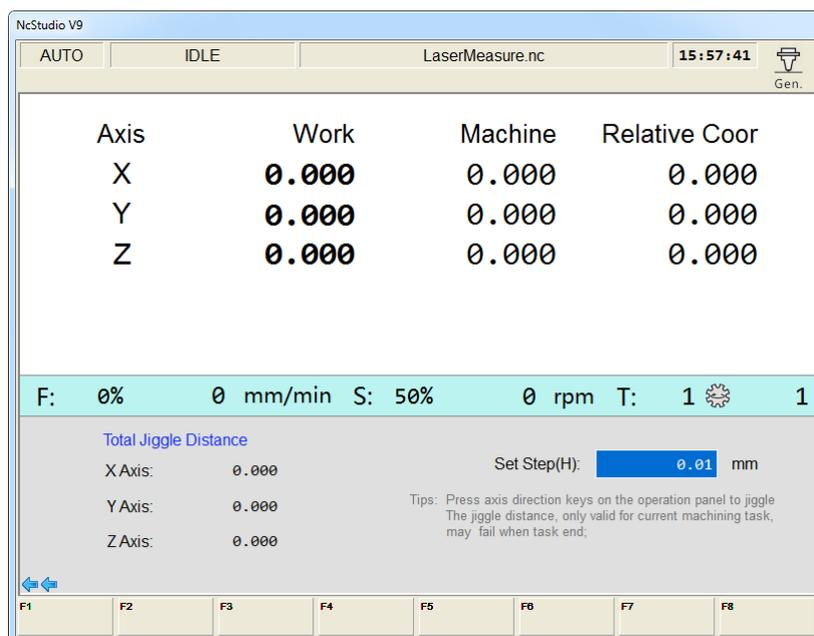
Fig. 3-101 Jiggle setup
