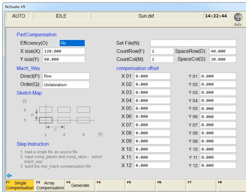
Fig. 3-67 Workpiece compensation interface
