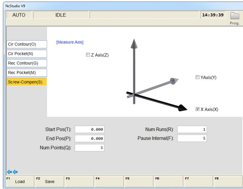
Fig. 3-77 Screw compensation screen
