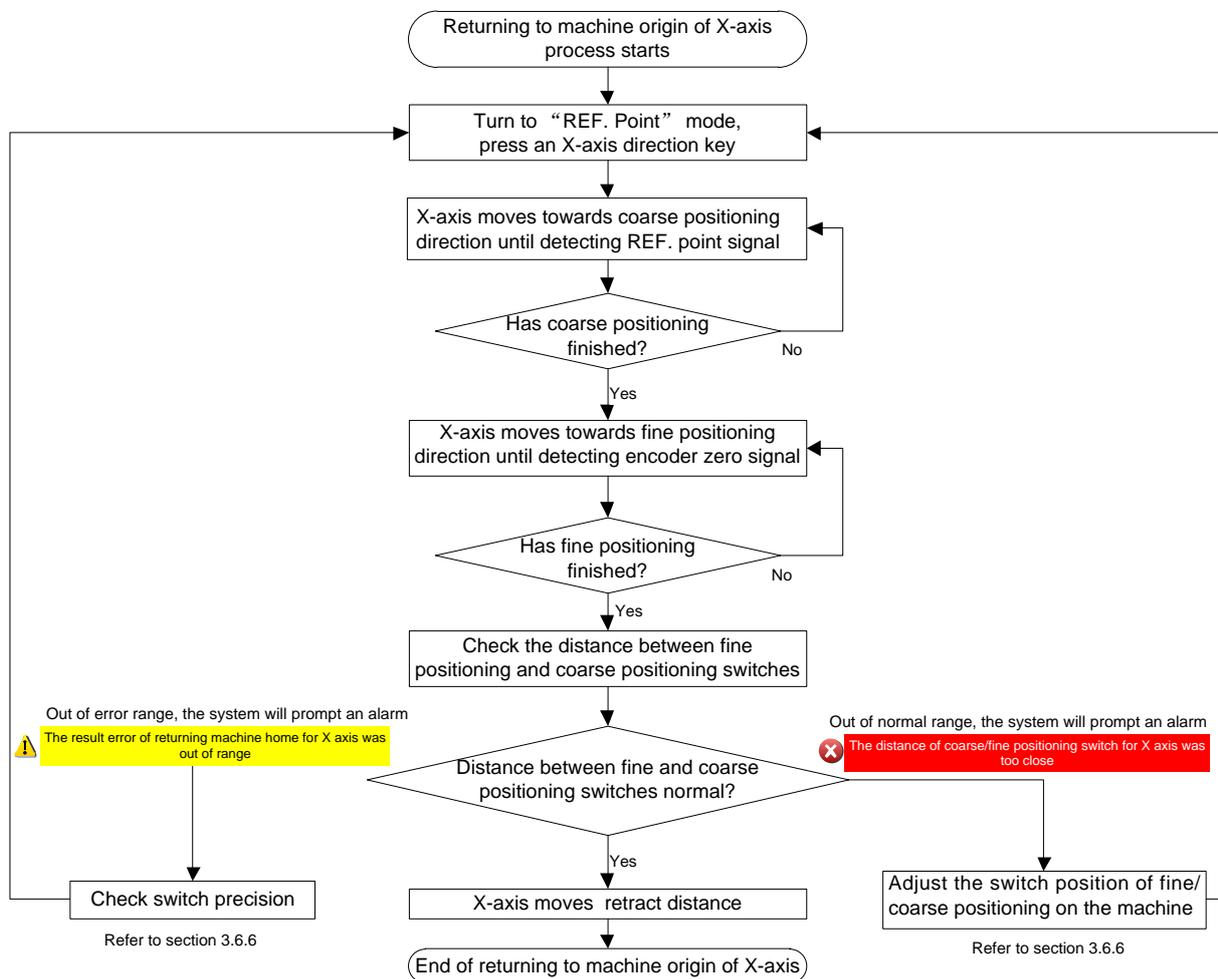
Fig. 3-9 The process of returning to machine origin (X-axis)
