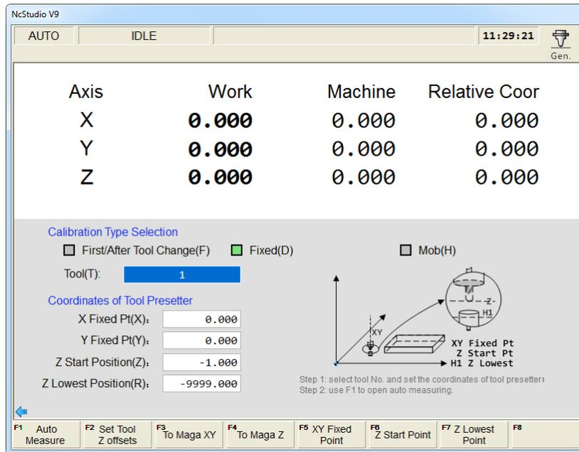
Fig. 3-35 Fixed calibration sub-screen
