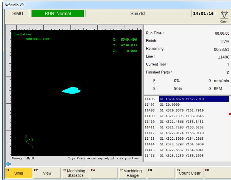
Fig. 3-59 Simulation and Track window
