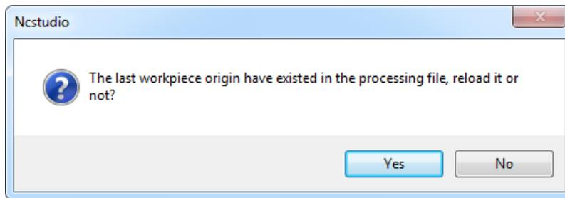
Fig. 3-43 Dialog box whether to reload existing origin
