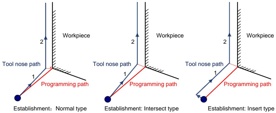
Fig. 3-64 Type to establish tool compensation
