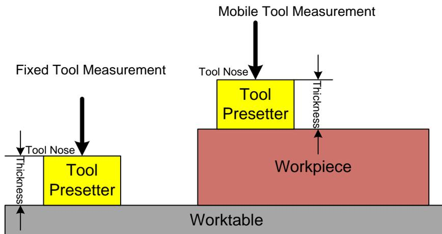
Fig. 3-27 Sketch map of using a tool presetter
