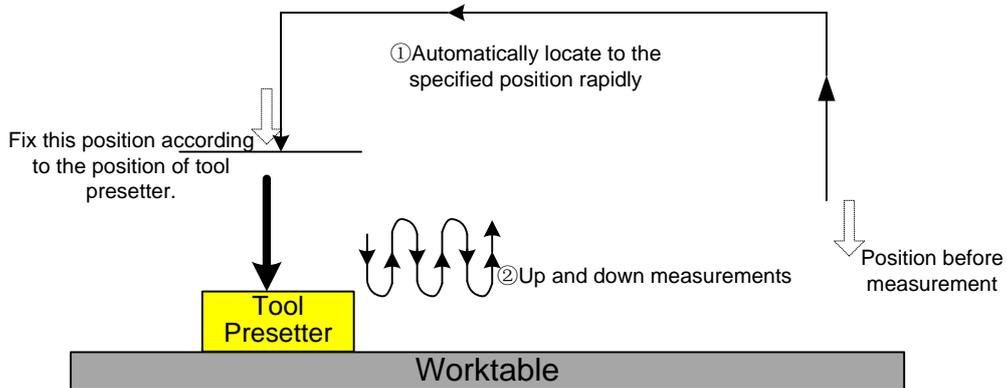
Fig. 3-32 The process of fixed calibration without encoder feedback function
