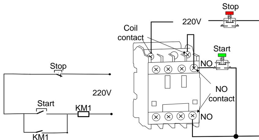
Fig. 2-6 Wiring diagram of electrical switch on 106 panel
