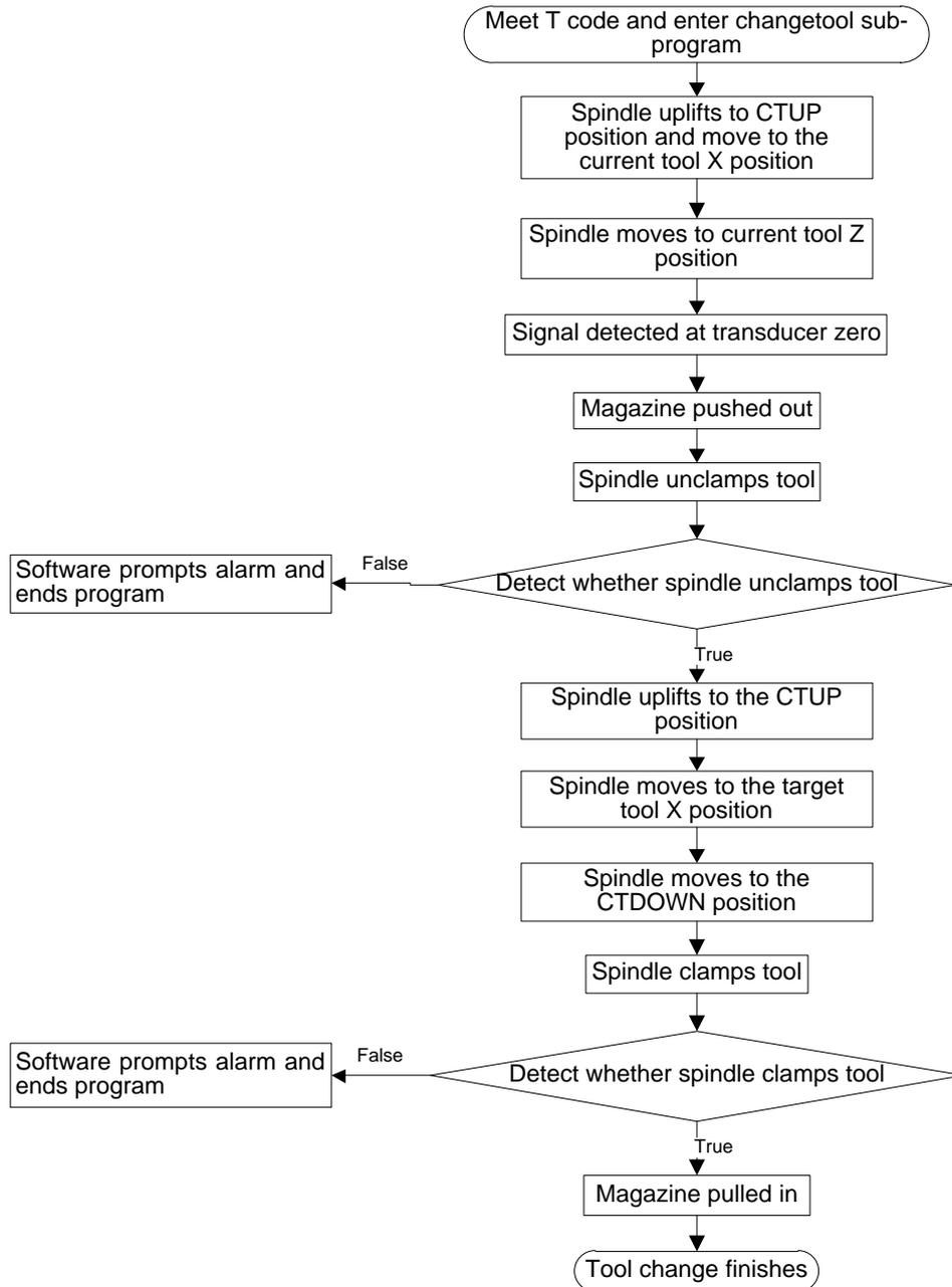
Fig. 3-107 Process of auto tool change for a linear tool magazine
