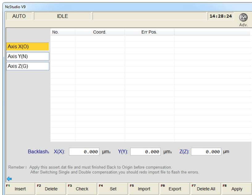
Fig. 3-71 Unidirectional compensation interface
