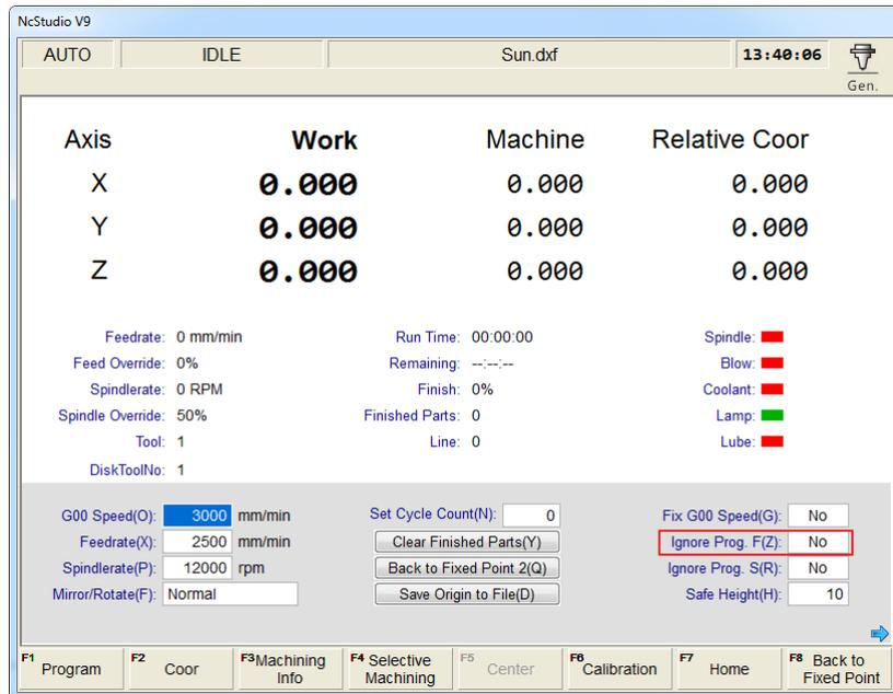
Fig. 3-53 Parameters setting zone-feedrate setting
