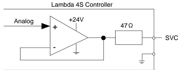
Fig. 2-5 Analog output signal circuit
