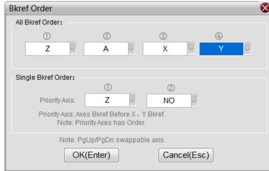
Fig. 3-14 All axes returning to the REF point
