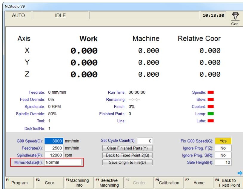
Fig. 3-103 Mirror and rotate setting on the main interface
