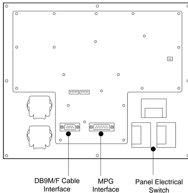
Fig. 1-16 Rear view of operation panel WH108A1
