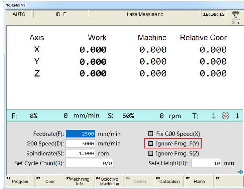
Fig. 3-24 Spindle speed setting on the new interface
