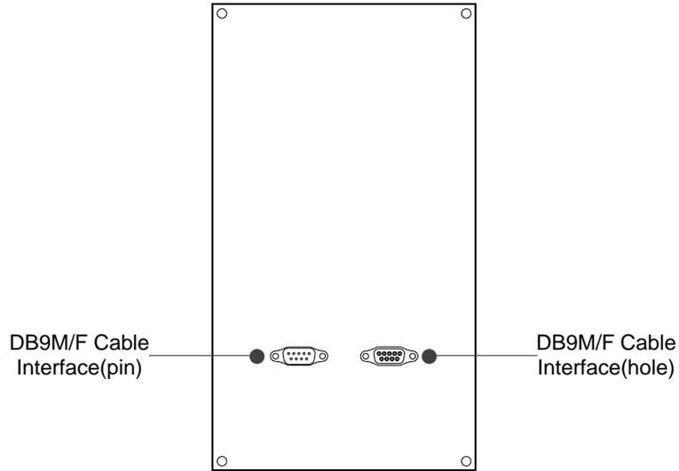
Fig. 1-13 Rear view of keypad panel KB1A1
