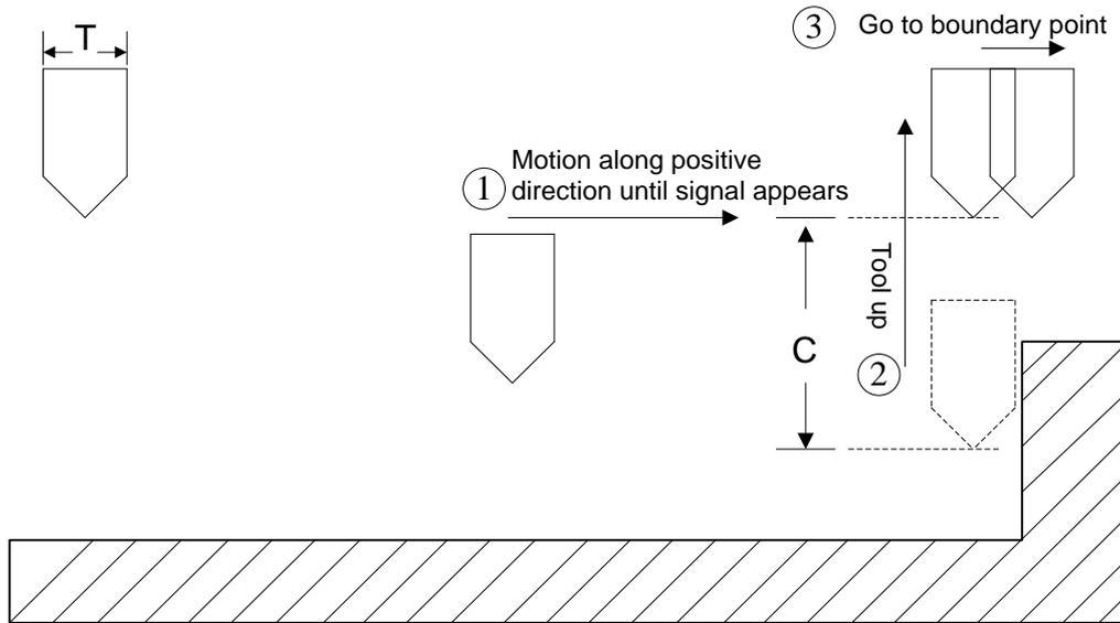
Fig. 3-52 Process of boundary center
