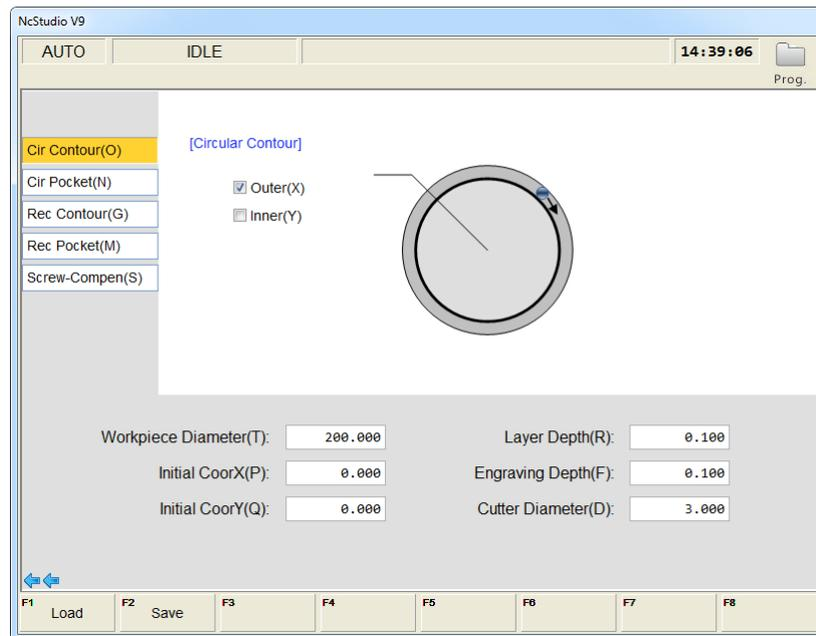
Fig. 3-76 Circular contour milling screen
