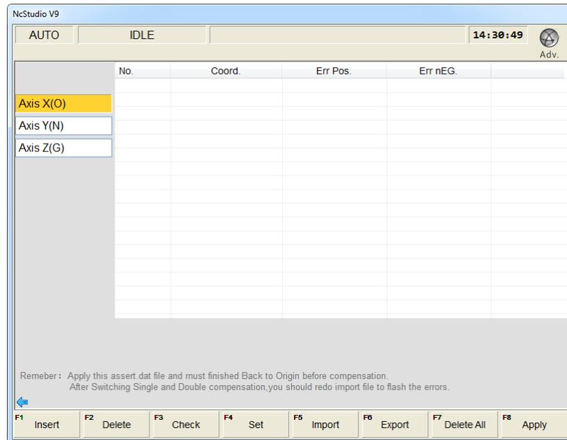
Fig. 3-72 Bidirectional compensation interface
