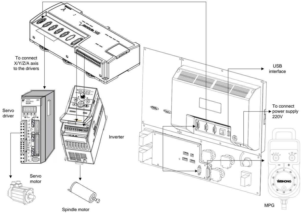
Fig. 1-17 Overall connection diagram of NK300BX-H
