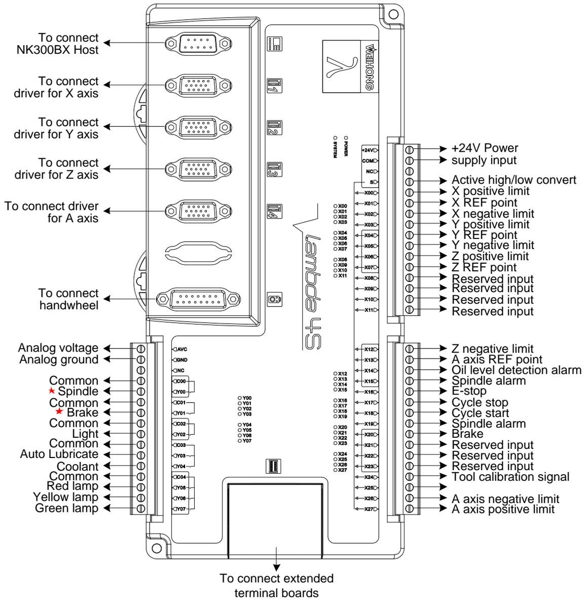
Fig. 2-8 Wiring diagram of Lambda 4S controller
