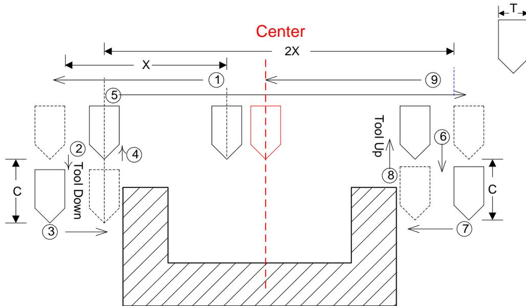
Fig. 3-50 The process of X outer center
