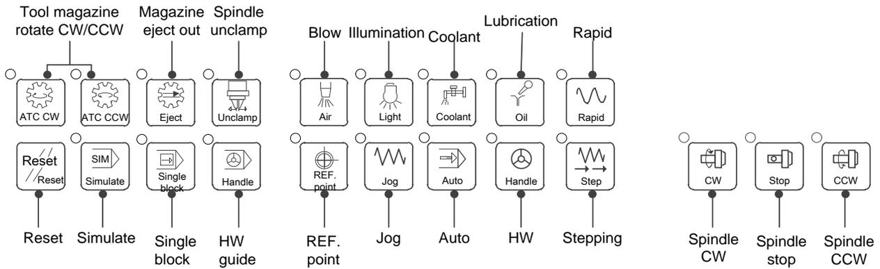
Fig. 1-15 Auxiliary functional keys and mode selection keys
