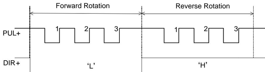
Fig. 2-3 Pulse command output mode
