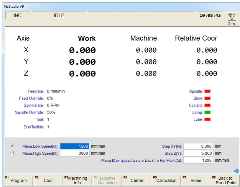
Fig. 3-56 Setting of jog speed and rapid jog speed
