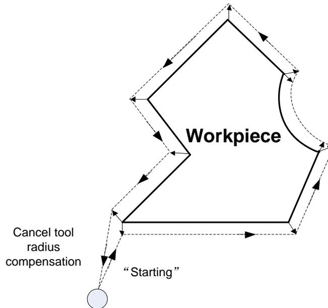
Fig. 3-63 Schematic Diagram for Tool Radius Compensation
