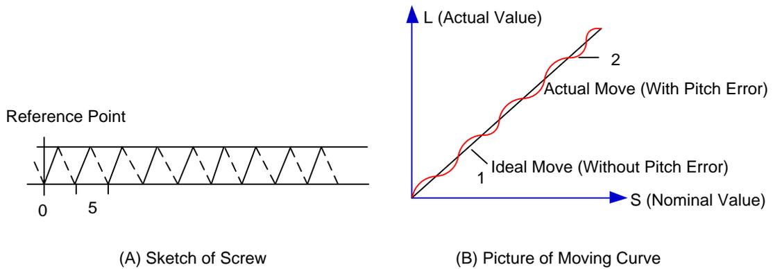
Fig. 3-69 Analysis of pitch error
