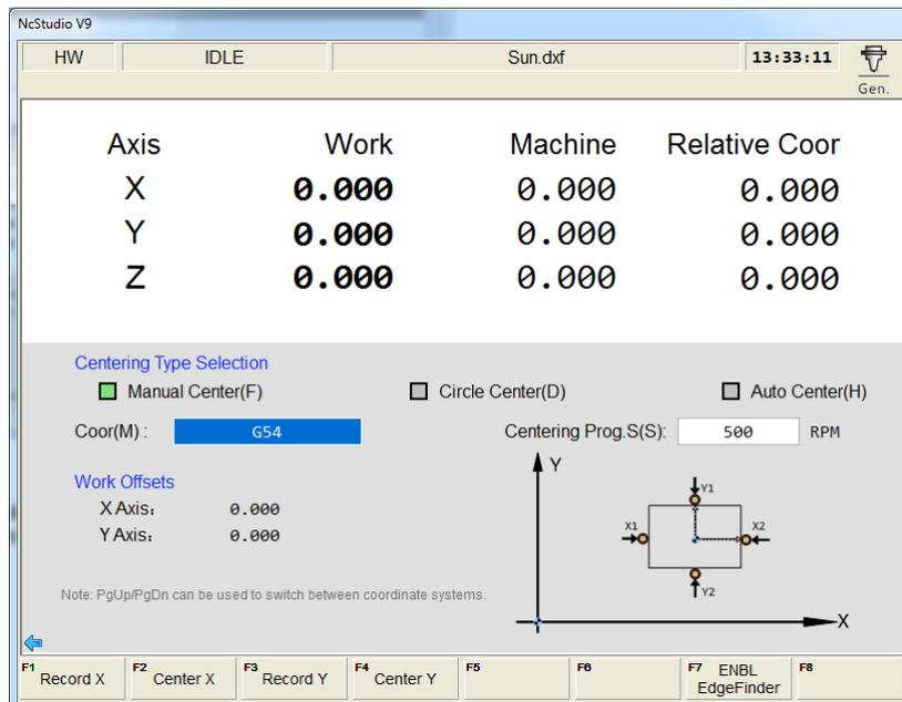
Fig. 3-47 Centering interface---Manual Center
