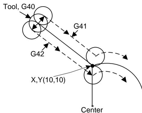
Fig. 3-66 Schematic diagram of tool compensation machining
