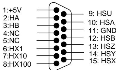
Fig. 2-14 Handwheel interface definition
