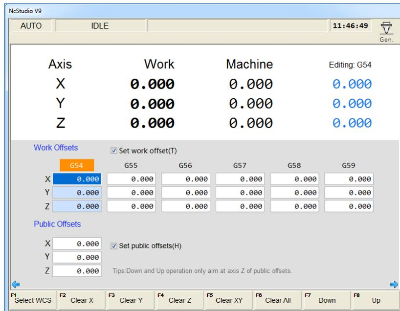
Fig. 3-41 Coordinate system management interface
