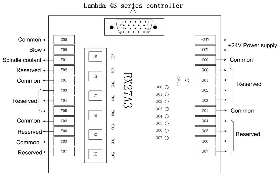
Fig. 2-12 Wiring diagram of terminal board EX27A3
