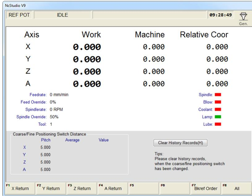
Fig. 3-12 Classic interface in REF mode---Four axes configuration
