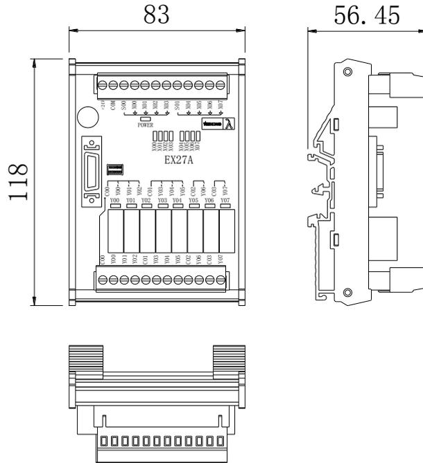
Fig. 2-11 Mounting Dimension of Terminal Board EX27A3
